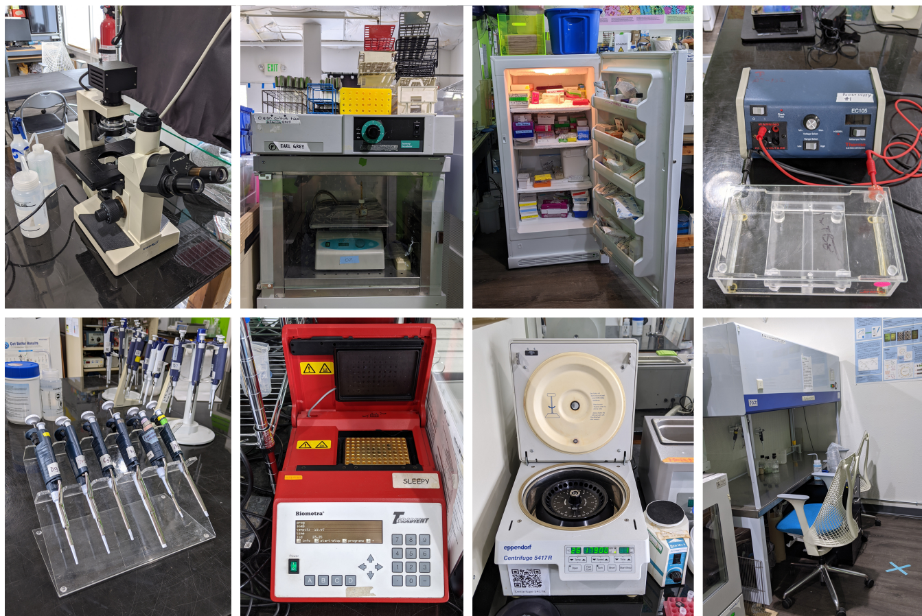
Figure 4: Some of the specialized equipment commonly found in many of the community biolabs in our sample. Nearly all of our labs acquired professional-grade equipment through donations or secondhand purchases. These photos were all taken at SOUND BIO LAB. Top row, left to right: Light Microscope; Incubator with orbital shaker positioned inside; Fridge; Gel electrophoresis equipment. Bottom row, left to right: Set of micropipettes; Thermocycler; Benchtop microcentrifuge; Laminar flow hood.
