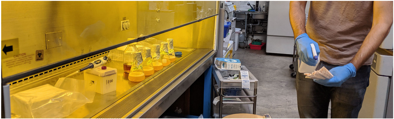
Figure 1: Biosafety cabinet, pipette, and materials for a DIYbio project in a community biolab.
