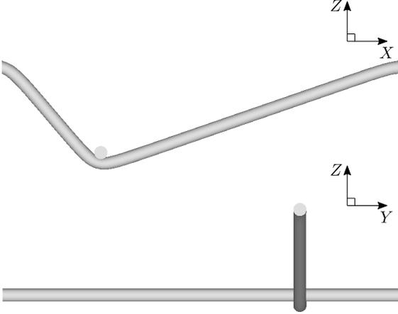
**Fig. 21:** Sliding contact between two initially straight beams (case 1): Final deformed configuration in the case of rigid slave (upper) beam. For the discretization of the beam axis, we use B-spline basis functions with  $p = 3$ , and  $n_{\text{el}} = 80$  and  $n_{\text{el}} = 160$  for the slave and master bodies, respectively. The chosen penalty parameter is  $\epsilon_{\text{N}} = 20E/L_0$ .
