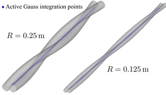
**Fig. 29:** Twisting of a wire strand (two wires): The final deformed configurations for two cases of the initial cross-section's radius:  $R = 0.25$  m, and  $R = 0.125$  m. The blue dots indicate the active surface Gauss integration points. In both cases, we use  $p = 3$ ,  $n_{\text{el}} = 40$ , and  $\epsilon_N = 10^2 E/L_0$ .
