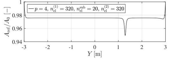
(a) Ratio between the cross-section area of the reference solution and the initial solution
