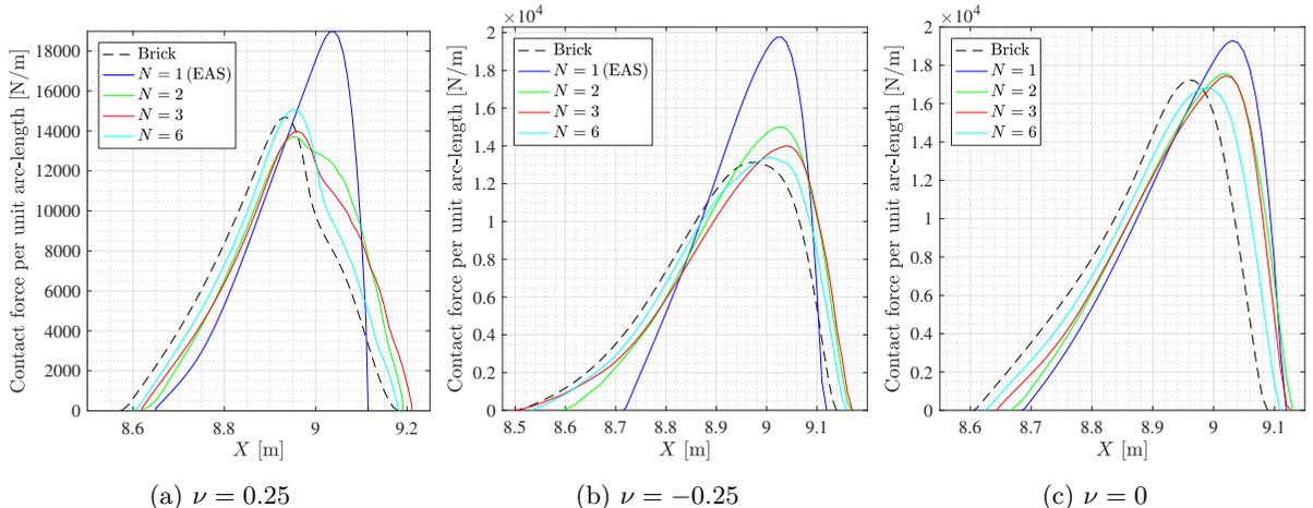
**Fig. 13:** Lateral contact of a straight beam: Comparison of the distribution of the contact force per unit initial arc-length (i.e.,  $r_N$  from Eq. (124)) along the beam axis for the final deformed configuration (i.e.,  $\lambda_{\text{load}} = 1$ ) for three values of Poisson’s ratio. We use brick elements with  $\text{deg.}=(3, 3, 3)$ ,  $n_{\text{el}} = 80 \times 10 \times 10$ , and beam elements with  $p = 3$  and  $n_{\text{el}} = 80$ .
