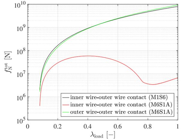
**Fig. 35:** Twisting of a wire strand (seven wires): Change of the average of the total contact force from Eq. (123) between corresponding contact pairs. We use  $p = 3$ ,  $n_{\text{el}} = 20$ , and  $\epsilon_N = 10E/L_0$ .
