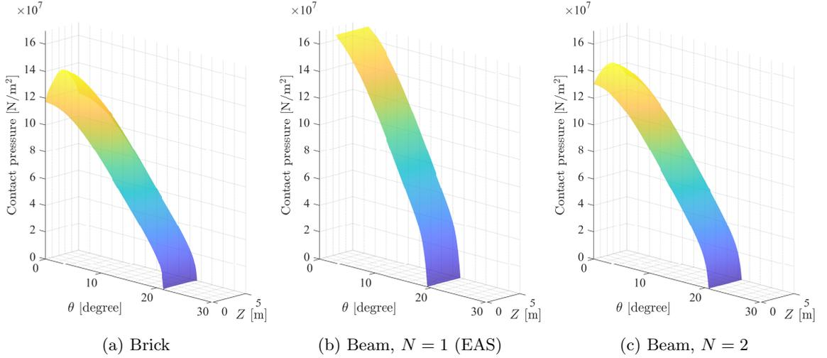
**Fig. 17:** Lateral contact of a circular ring: Comparison of contact pressure distributions on the bottom surface in beam and brick element models. (a) We use brick elements of deg. = (4, 4, 4),  $n_{el} = 320 \times 4 \times 4$ , (b,c) and beam elements of  $p = 3$ , and  $n_{el} = 320$ .
