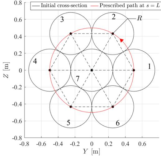
**Fig. 33:** Twisting of a wire strand (seven wires): Initial configurations of strands in the cross-sectional  $Y$ - $Z$  plane, and the prescribed circular paths at the ends ( $s = L$ ), indicated by the red circle.
