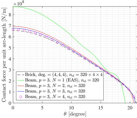
**Fig. 18:** Lateral contact of a circular ring: Comparison of the distribution of the contact force per unit initial arc-length, i.e.,  $r_N$  from Eq. (124), at the bottom surface in beam and brick element solutions. We use brick elements of deg. = (4, 4, 4),  $n_{el} = 320 \times 4 \times 4$ .
