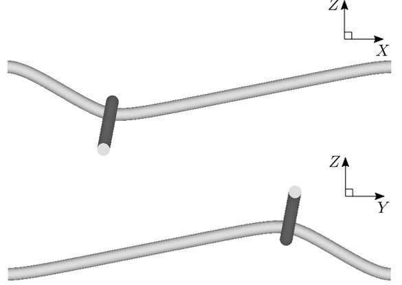
**Fig. 25:** Sliding contact between two initially straight beams (case 2): For the discretization of the beam axis, we use B-spline basis functions with  $p = 3$ , and  $n_{\text{el}} = 160$  for both the slave and master bodies. The chosen penalty parameter is  $\epsilon_N = 10^2 E/L_0$ .
