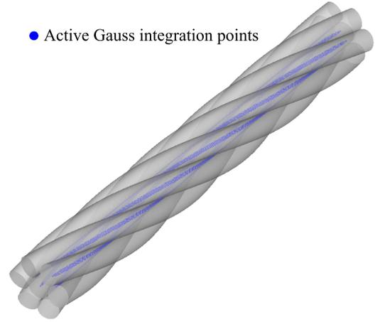
**Fig. 34:** Twisting of wire strands (seven wires): The final deformed configuration. We use  $p = 3$ ,  $n_{\text{el}} = 20$ , and  $\epsilon_N = 10E/L_0$ , and select the outer beams as the slave bodies, and the inner beam as the master body (M1S6). The blue dots indicate the active surface Gauss points.
