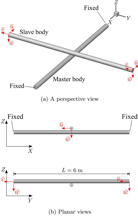
**Fig. 20:** Sliding contact between two initially straight beams: Initial configuration and boundary conditions. The prescribed displacements in  $X$ -,  $Y$ -, and  $Z$ -directions at the ends of the upper beam are denoted by  $\bar{u}$ ,  $\bar{v}$ , and  $\bar{w}$ , respectively, and chosen as  $\bar{u} = \bar{v} = \bar{w} = -1.5$  m.
