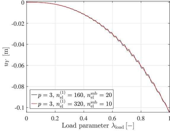
**Fig. 26:** Contact between two initially straight beams (case 2):  $Y$ -displacement at the center of axis ( $s = L/2$ ) in the master beam for two different discretization. It should be noted that those two cases have the same total number of Gauss integration points for the evaluation of the contact integral on the slave body. In all cases, we use  $m_{\text{el}}^{\text{sub}} = 100$ .
