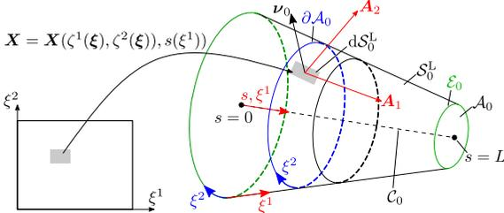
**Fig. 6:** Parameterization of the beam's initial lateral boundary surface  $\mathcal{S}_0^L$ . Note that the initial axis is parameterized by the same coordinate  $\xi^1$  used for the longitudinal direction of the lateral boundary surface.
