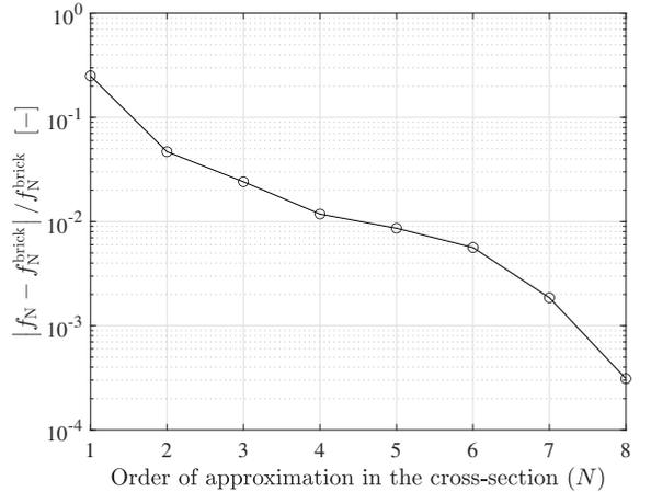
**Fig. 19:** Lateral contact of a circular ring: Convergence of the relative error in total contact force between the beam ( $f_N$ ) and brick ( $f_N^{\text{brick}}$ ) element solutions, with increasing the order of approximation in the cross-section ( $N$ ). We use brick elements of deg. = (4, 4, 4),  $n_{el} = 320 \times 4 \times 4$ , and beam elements of  $p = 3$ , and  $n_{el} = 320$ .
