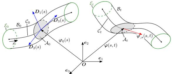
**Fig. 1:** A schematic illustration of the beam kinematics in the initial and current configurations. Note that the initial cross-section ( $\mathcal{A}_0$ ) is assumed planar; however, the current one ( $\mathcal{A}_t$ ) is not always planar due to out-of-plane deformations for  $N \geq 2$  in Eq. (2).
