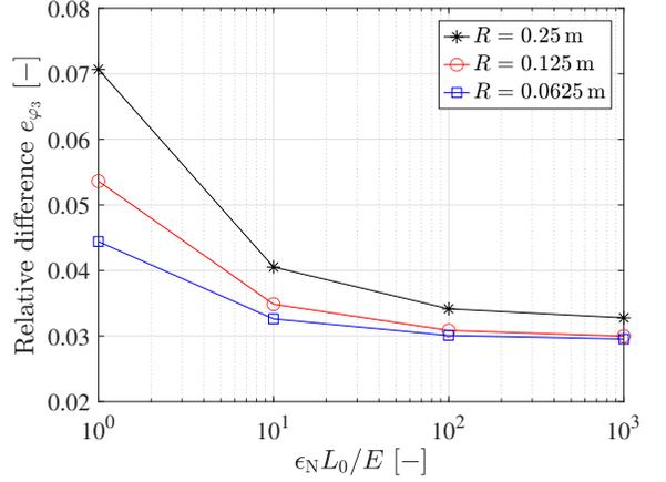
**Fig. 31:** Twisting of a wire strand (two wires): The relative  $L^2$ -norm of Eq. (132) versus the normal contact penalty parameter. We use  $N = 1$  combined with the EAS method, and  $p = 3$  and  $n_{\text{el}} = 40$ .
