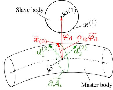
**Fig. 8:** A geometrical approach of selecting an initial guess  $\bar{\mathbf{x}}_{(0)} \equiv \mathbf{x}^{(2)}(\bar{\xi}_{(0)})$  in the local contact search as the intersection of the vector  $\alpha_{\text{ig}} \widetilde{\boldsymbol{\varphi}}_d$  with the boundary of the projected cross-section  $\partial\widetilde{\mathcal{A}}_t$ .
