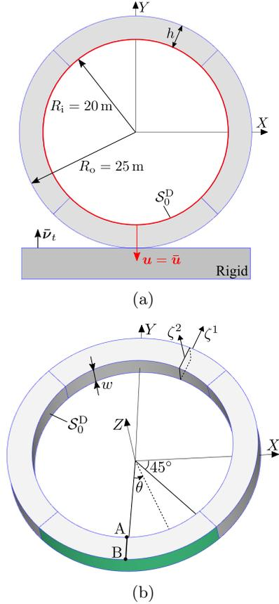
**Fig. 15:** Lateral contact of a circular ring: (a) undeformed configuration and prescribed displacement boundary condition at the inner surface  $S_0^D$ . The blue lines indicate the division of the domain into four parts due to modeling the ring exactly with four NURBS curves. (b) The two cross-sectional coordinates  $\zeta^1$  and  $\zeta^2$  are aligned with the radial, and  $Z$ -directions, respectively. In this problem, we consider contact only on the green-colored surface.
