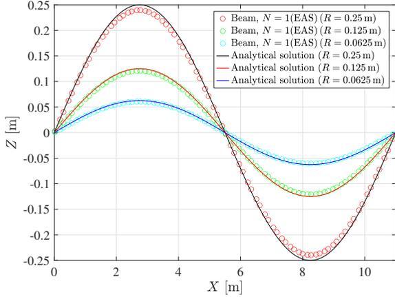
**Fig. 30:** Twisting of a wire strand (two wires): Comparison of the final deformed configuration of the axis of the master body in the  $X$ - $Z$  plane for three different values of the initial cross-section radius:  $R = 0.25$  m,  $0.125$  m, and  $0.0625$  m. Solid lines indicate the analytical solutions of Eq. (131). In all cases, we use  $p = 3$ ,  $n_{\text{el}} = 40$ , and  $\epsilon_N = 10^2 E/L_0$ .
