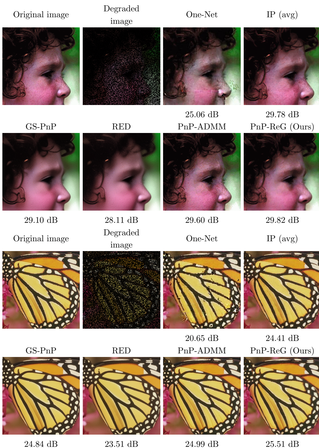
Figure 5. Visual comparison of pixel-wise inpainting results with known pixel rate of p = 20\% , obtained with the projection operator (One-Net) [44], the Implicit Prior (IP) of [27], GS-PnP [26], RED [45], PnP-ADMM with the denoiser of [62] and our PnP-ReG method.
