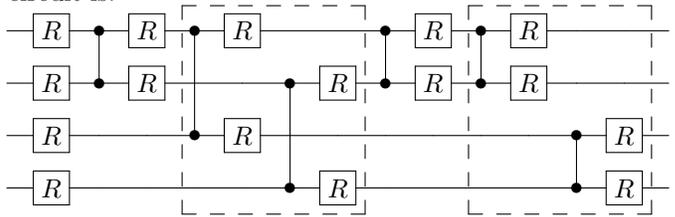
The two pairs of steps that can each be parallellized are shown by the dashed boxes.
