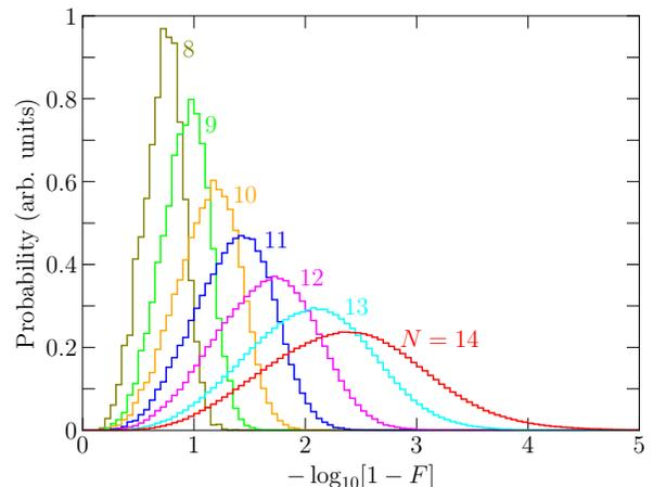
FIG. 6: Histograms of fidelity  $F$  values for all the possible CNOT gate configurations for the problem of synthesizing a three-qubit unitary operator using two-qubit CNOT gates and single-qubit gates. The olive, green, orange, blue, magenta, cyan and red lines correspond, respectively, to  $N = 8, 9, 10, 11, 12, 13$  and  $14$ . All the data in this figure were obtained using  $10^3$  optimization iterations.
