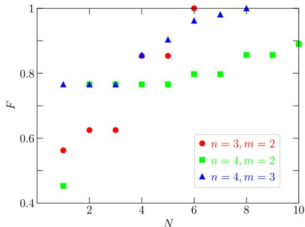
FIG. 7: The maximum achievable fidelity  $F$  as a function of quantum circuit size  $N$  for synthesizing a multi-qubit Toffoli gate. The red circles are for the well-known case of synthesizing a three-qubit Toffoli gate from two-qubit CNOT gates. The green squares are for the case of synthesizing a four-qubit Toffoli gate from two-qubit CNOT gates. The blue triangles are for the case of synthesizing a four-qubit Toffoli gate from three-qubit Toffoli gates.
