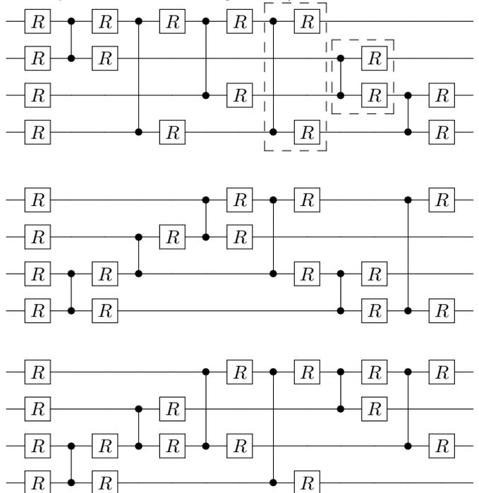
Each one of these quantum circuits can be used to generate 23 other equivalent ones by qubit permutations. Furthermore, the fourth and fifth CZ gates in the first quantum circuit operate on different qubits and there-
