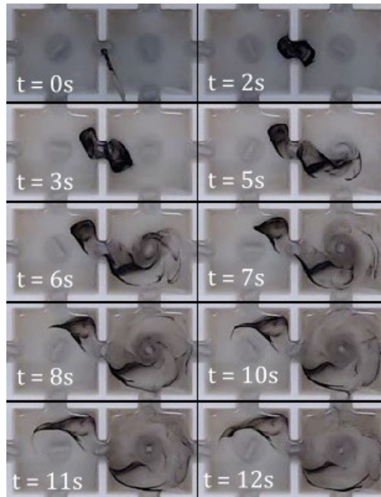
Fig. S21: Hydrodynamic tests towards asymmetric coupling. Shows snapshots at a different time demonstrating symmetric coupling between the two cells.
