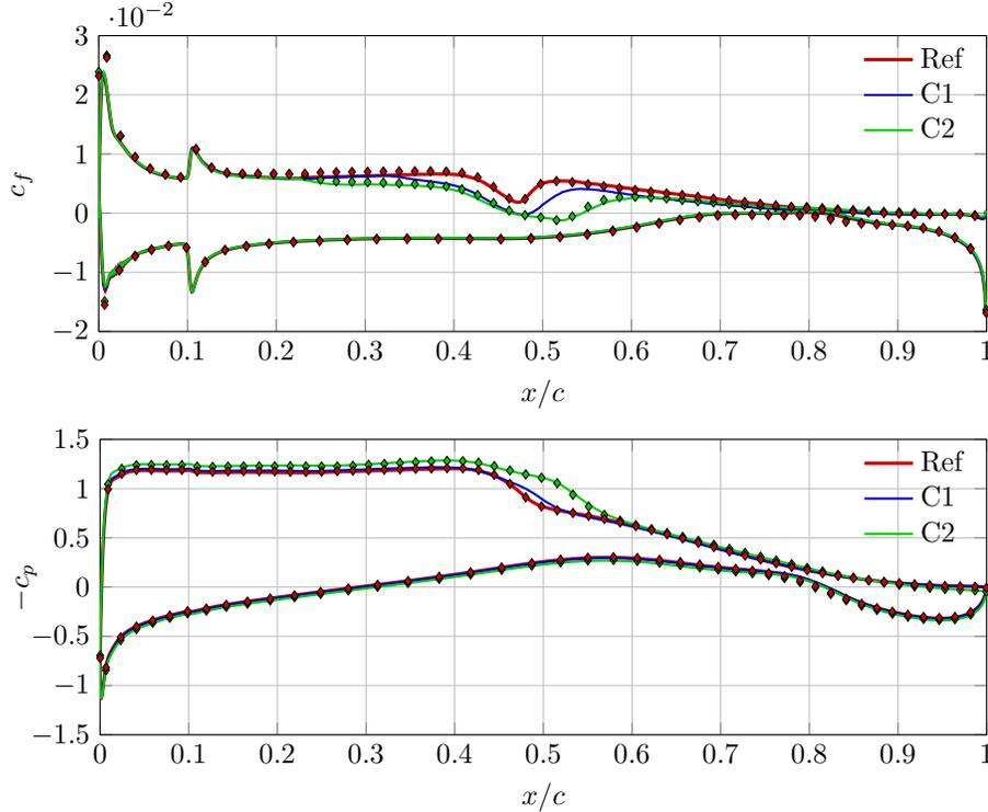
FIGURE 4. Mean friction coefficient  $c_f$  (top) and mean pressure coefficient  $c_p$  (bottom). Symbols denote the uncontrolled and C2 cases computed on the finer mesh. Note that green and red symbols almost overlap on the pressure side.
