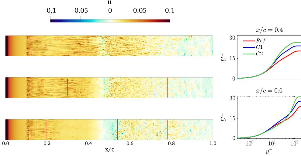
FIGURE 3. Instantaneous chord-wise velocity at the first grid point off the wing surface over the suction side, for uncontrolled (top), C1 (middle) and C2 (bottom) flow cases. Red lines mark the boundaries of the actuated region, and green lines the position of the shock. The panels on the right plot the mean velocity profile in local wall units upstream and downstream of the shock.
