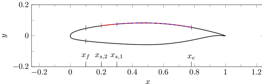
FIGURE 1. Geometry of the V2C airfoil. Forcing is applied at  $x_f$  (on both sides) to initiate transition.  $x_s$  and  $x_e$  denote start and end of the suction-side actuated region for cases C1 (blue dashed line) and C2 (red continuous line).
