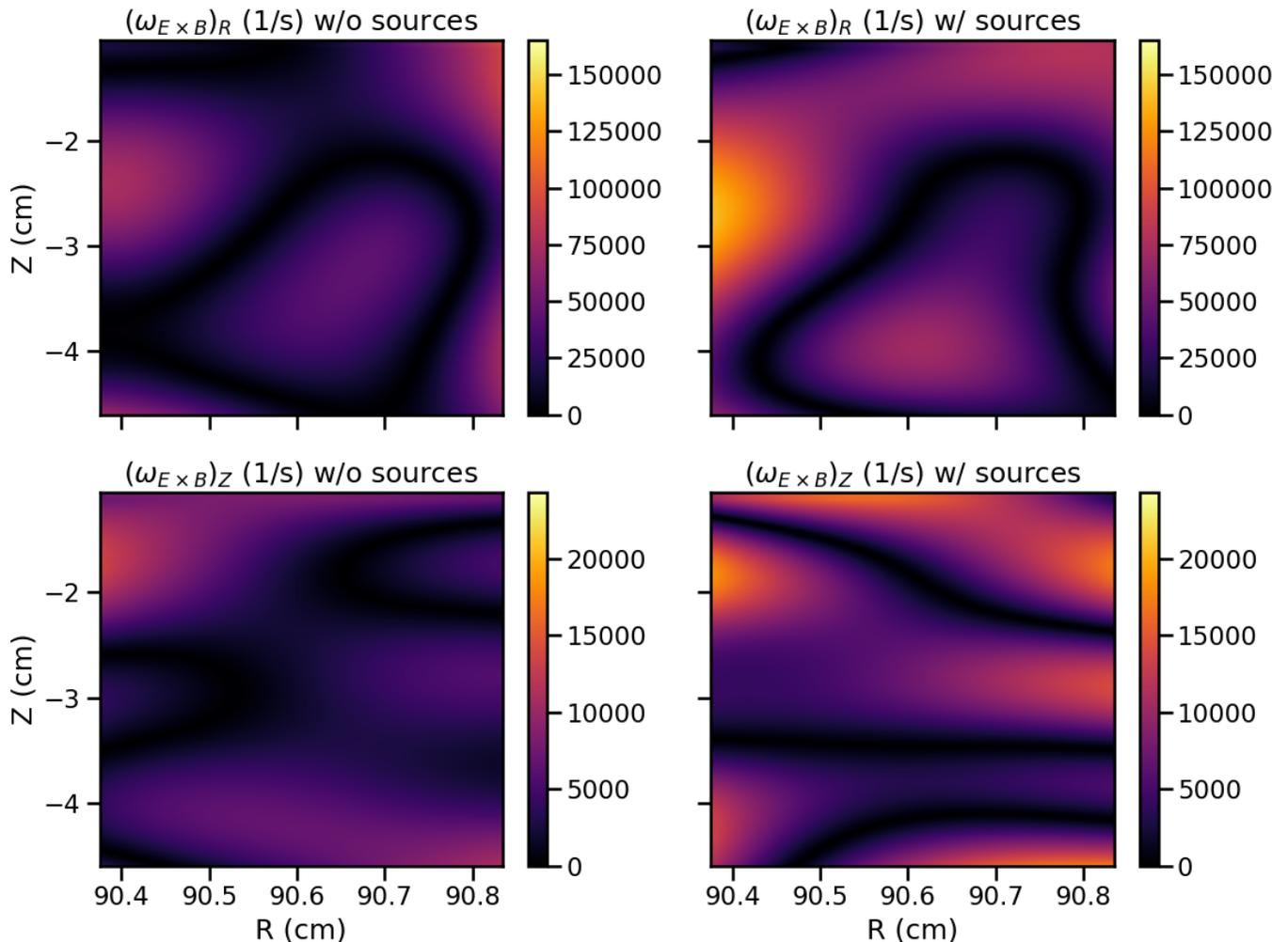
FIG. 3. Visualizations of the radial and vertical turbulence shearing rates predicted by drift-reduced Braginskii theory in discharge 1120711021 at  $t = 1.312886$  s on Alcator C-Mod under the assumption of axisymmetry with a toroidal field. The plots consider no sources (left) and, alternatively, neutral sources to account for time-dependent ionization of HeI (right).
