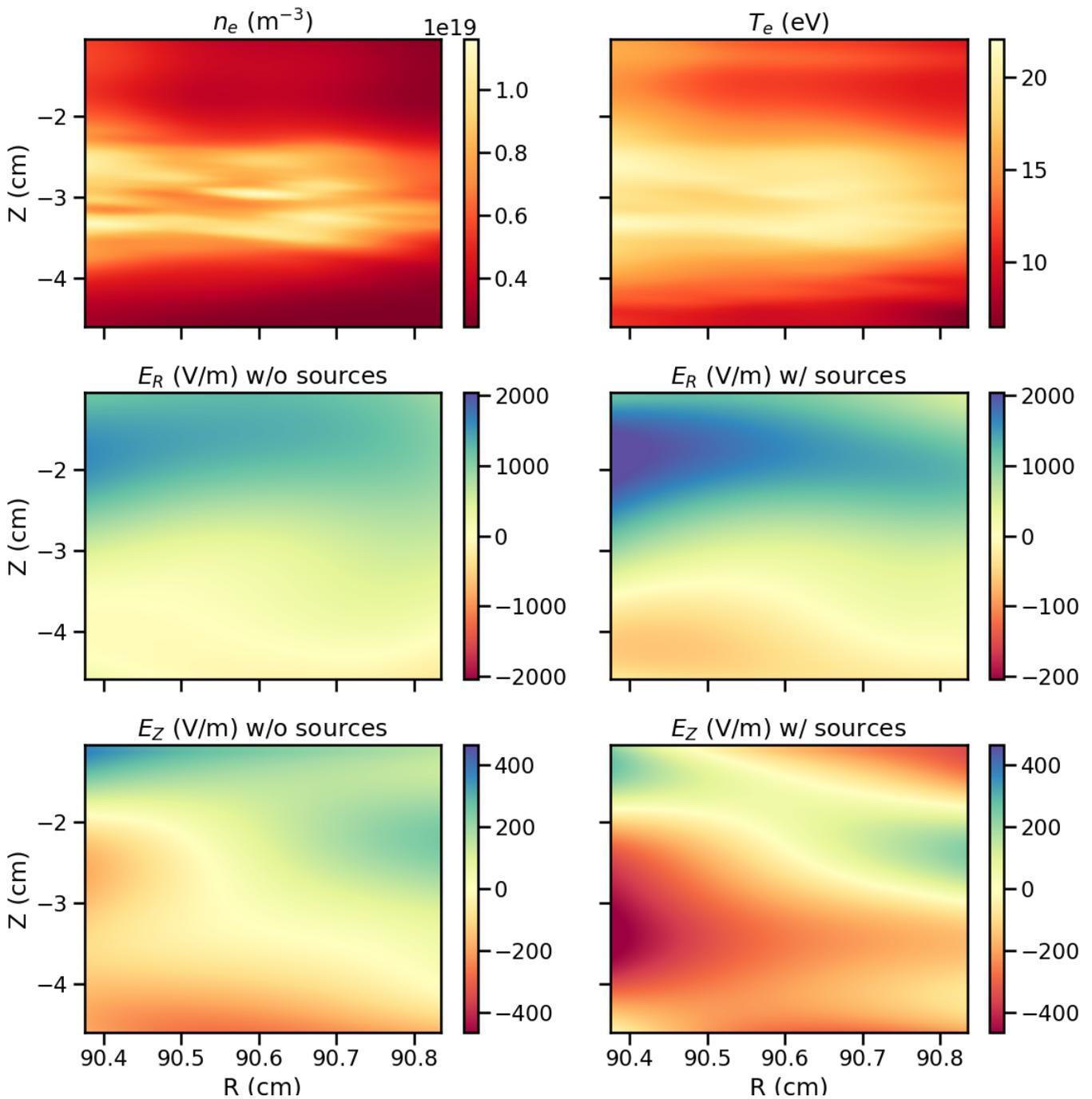
FIG. 1. The 2-dimensional  $n_e$  and  $T_e$  (top row) come from experimental GPI of discharge 1120711021 on Alcator C-Mod at  $t = 1.312886$  s [2]. The  $E_R$  and  $E_Z$  are inferred from drift-reduced Braginskii theory using these experimental  $n_e$  and  $T_e$  according to the outlined deep learning framework [1] in the limiting cases of with (i.e. scaling factor of  $n_0^* = 10^{19} \text{ m}^{-3}$ ) and without (i.e.  $n_0^* = 0$ ) HeI sources in the physical equations.
