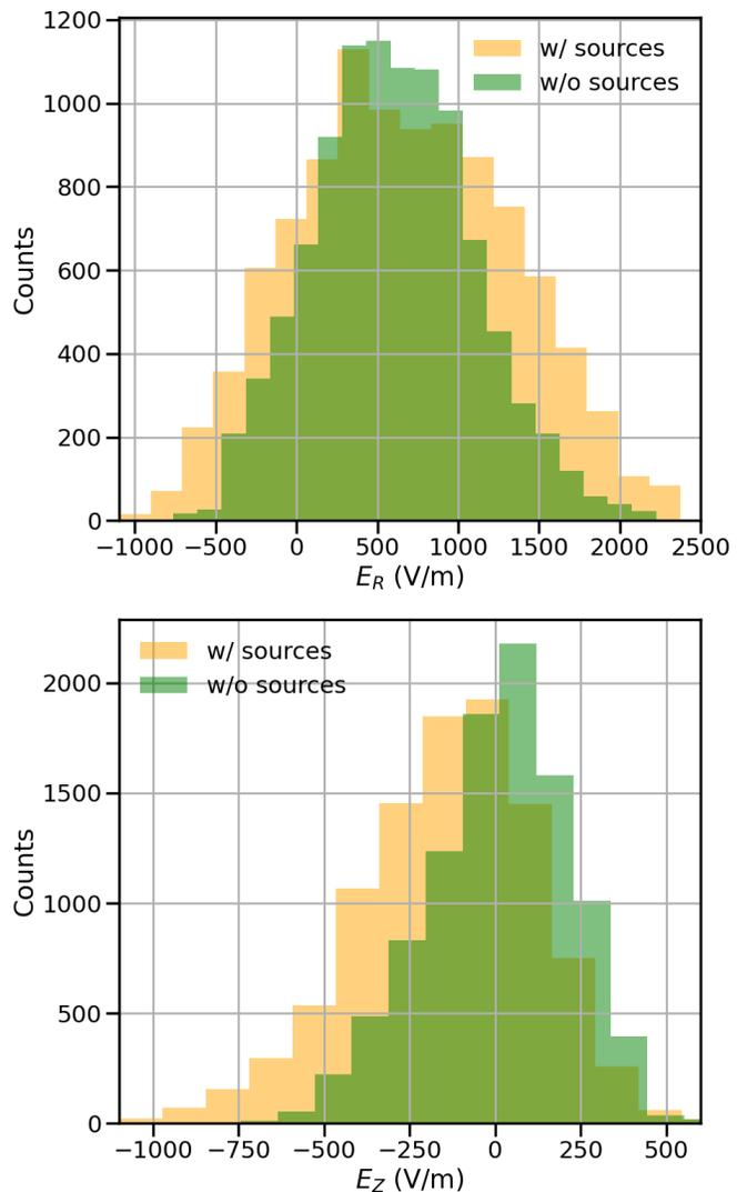
FIG. 2. Histograms of  $E_R$  and  $E_Z$  consistent with drift-reduced Braginskii theory in a toroidal axisymmetric geometry evaluated at the GPI pixels from  $90.3 < R$  (cm)  $< 90.9$ ,  $-4.6 < Z$  (cm)  $< -1.0$ , and  $1.312799 < t_{GPI}$  (s)  $< 1.312896$  in discharge 1120711021 on Alcator C-Mod.
