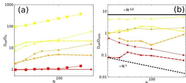
FIG. 9: Diffusion coefficient of the polymer center of mass  $D_{eff}$  as a function of the polymer length for three different  $Pe$  values 0 (red), 0.1 (orange) and 1 (yellow). (a)
