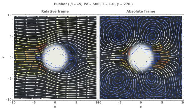
FIG. 11: Pusher swimming to the right with  $v_p \approx 0.4$ ,  $v \approx 3.236$ ,  $Re \approx 0.1236$ ,  $Pe \approx 659.58$ . Here we can achieve this lower Reynolds number because we choose the friction coefficient of the DPD solvent as  $\gamma^{ss} = 270$ . **Left:** frame moving with the colloid. **Right:** lab frame.
