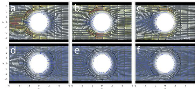
FIG. 4: Solvent flow fields of the colloid confined in a cylindrical channel ( $R_{cyl} = 3.5$ ) in the lab frame (bottom row) and moving with the colloid (top row), for the pusher (a, d), neutral (b, e) and puller (c, f) squirmer. Here the colloid radius is  $R_c = 2$  and  $F_p = 50$ . These values produce  $Pe \approx \{90, 76, 61\}$  and  $Re \approx \{3.9, 3.3, 2.7\}$  for the pusher, neutral and puller squirmer respectively.
