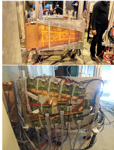
FIG. 10: Integration of the cooling plate in the test beam experimental setup. Upper: Detector side, Lower: FEB side.
