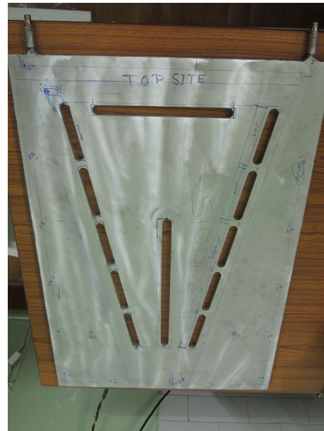
FIG. 8: Sample cooling plate after fabrication using technique II.
