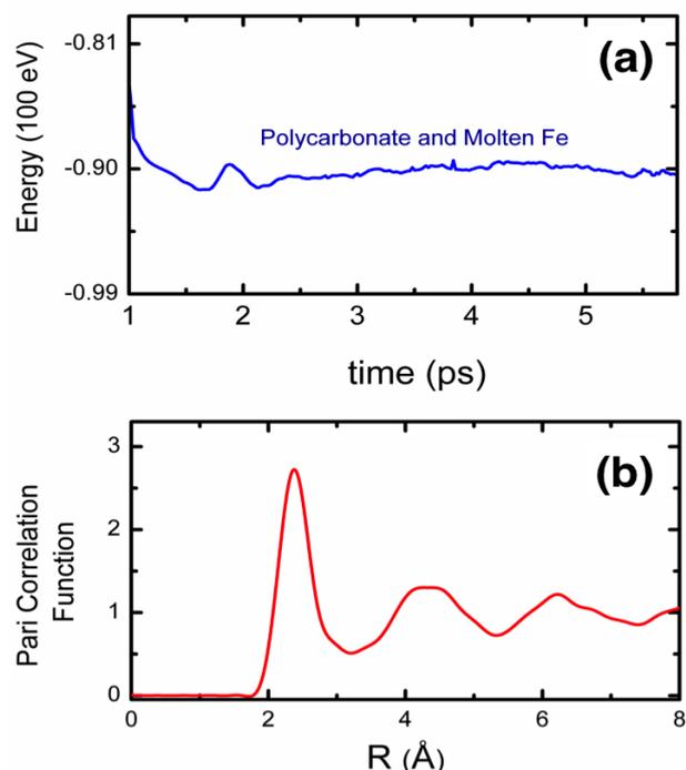
**Figure 1.** (a) Energy fluctuations during molecular dynamics simulation of interacting polycarbonate monomer and molten Fe system. (b) Pair correlation function of molten Fe at 1823 K obtained from *ab initio* molecular dynamics simulation.
