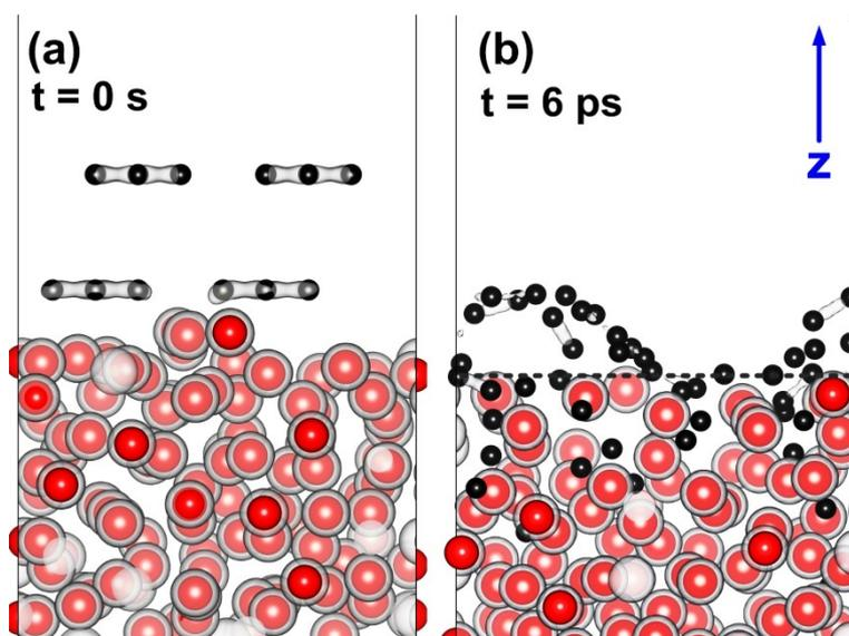
Figure S1. The decomposition and dissolution of the graphite sheets in molten iron at  $T = 1823$  K ( $\sim 1550$  °C). The red and black balls represent Fe and C atoms respectively. The gray shade surrounding the atoms represents electronic charge density around each atom which also indicates the atomic bonds. In (b) one can see the disappearance of C–C bonds as the graphite sheets are dissolved in molten Fe.
