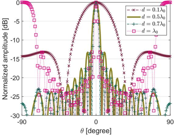
Fig. 1. Zero-time cut of the FITB (9).
