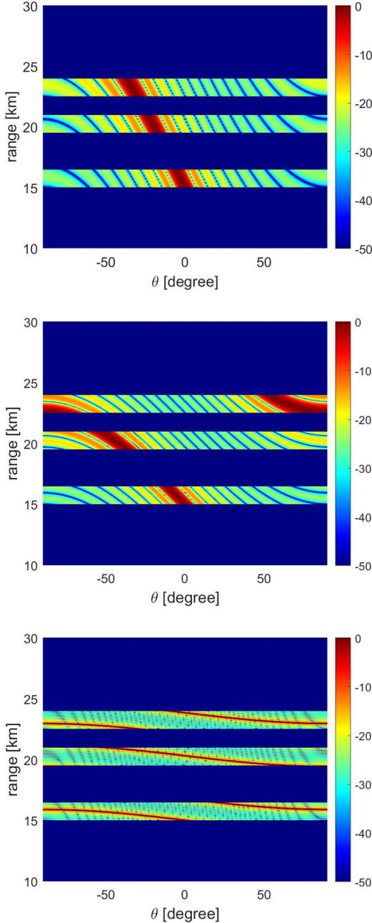
Fig. 2. Illustration of the FDA array factor (10) at the observed instant  $t = 50 \mu\text{s}$ ,  $t = 65 \mu\text{s}$  and  $t = 75 \mu\text{s}$  in the existing FDA transmit beampattern studies. (a)  $\Delta f = 10 \text{ kHz}$ . (b)  $\Delta f = 20 \text{ kHz}$ . (c)  $\Delta f = 170 \text{ kHz}$ .
