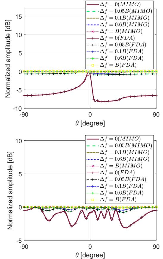
Fig. 6. Comparison of the FGTB and co-located MIMO transmit beampattern, with (a) uniform transmit weight  $\mathbf{w} = \mathbf{1}_M$  with  $\mathbf{1}_M$  being  $M \times 1$  vector of ones; (b) random transmit weight  $w_m = e^{j2\pi c_m m}$ ,  $m = 1, \dots, M-1$  with  $0 \leq c_m \leq 1$  being random number.
