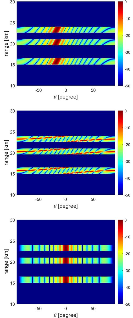
Fig. 3. Illustration of the proposed FITB (9) at the observed instant  $t = 50 \mu\text{s}$ ,  $t = 65 \mu\text{s}$  and  $t = 75 \mu\text{s}$  with considering the time-range relation. (a)  $\Delta f = 10 \text{ kHz}$ . (b)  $\Delta f = 200 \text{ kHz}$ . (c)  $\Delta f = 0 \text{ kHz}$ .
