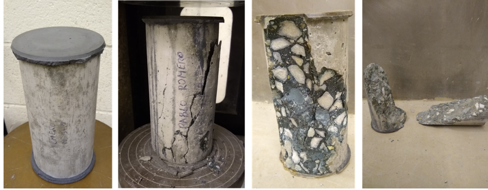
Fig. 9. Photographs of some concrete cylinders made according to novel formulations, undergoing laboratory testing for compressive strength.
