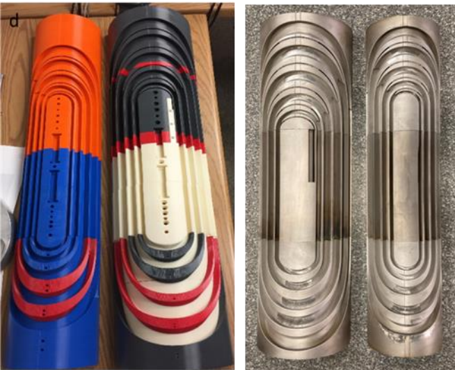
Fig. 2. Inner-layer and outer-layer plastic (left) and 316 stainless steel (right) parts for SMCT coils.
