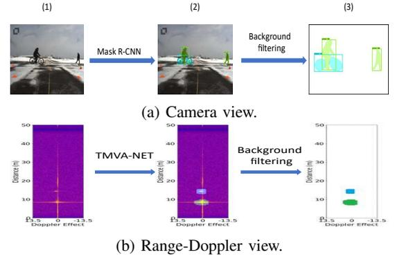
Fig. 2: A scene from CARRADA dataset from different views with their respective semantic segmentation, with a cyclist and a pedestrian. The blue mask in (b) represents the pedestrian while the green mask represents the cyclist.
