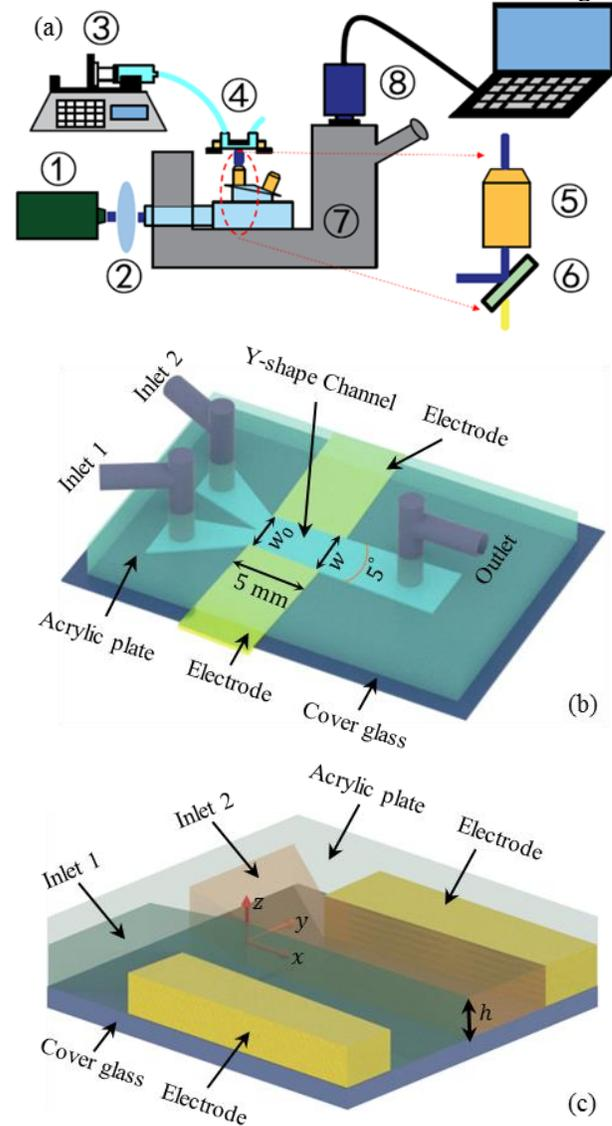
**Figure 1.** Schematic diagram of experimental system and microchannel. (a) Schematic diagram of the experimental system, includes ① 473 nm laser, ② lens set, ③ syringe pump, ④ EK micromixer, ⑤ dichroic mirror and bandpass filter, ⑥ objective lens, ⑦ inverted fluorescence microscope, ⑧ SCMOS camera. (b) Schematic diagram of the EK micromixer, and (c) the coordinate system in the EK micromixer.
