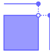
FIGURE 16. Local subdomain dof (o) corresponds to dofs (•) on two bilateral facets. For an element \tau_i \in \Lambda_i , the operation t_i = T_i^\top \tau_i adds up the values of the two trace dofs • to the local subdomain dof o. From t_i the original values of the two trace dofs cannot be recovered. Therefore \ker(T_i^\top) \neq \{0\} and \text{range}(T_i) \subsetneq \Lambda_i .
