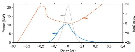
**Fig. 4 Mid-IR pulse characterisation.** Temporal intensity (blue-solid line) and phase (red-dashed line) profiles of the simulated mid-IR pulse at the fibre output. The pulse is centred at 3.1  $\mu\text{m}$  wavelength, and it has FWHM duration and peak power of 123 fs and 10.6 MW, respectively. At its Fourier limit, they are 67 fs and 20.4 MW (grey-dotted line).
