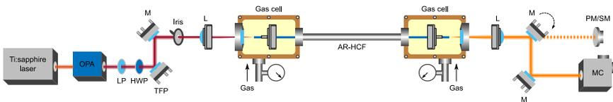
**Fig. 2 Experimental setup.** OPA, optical parametric amplifier; LP, long-pass filter; HWP, half-wave plate; TFP, thin-film polariser; PM, power meter; SM, spectrometer; MC, monochromator; M, mirror; L, lens.
