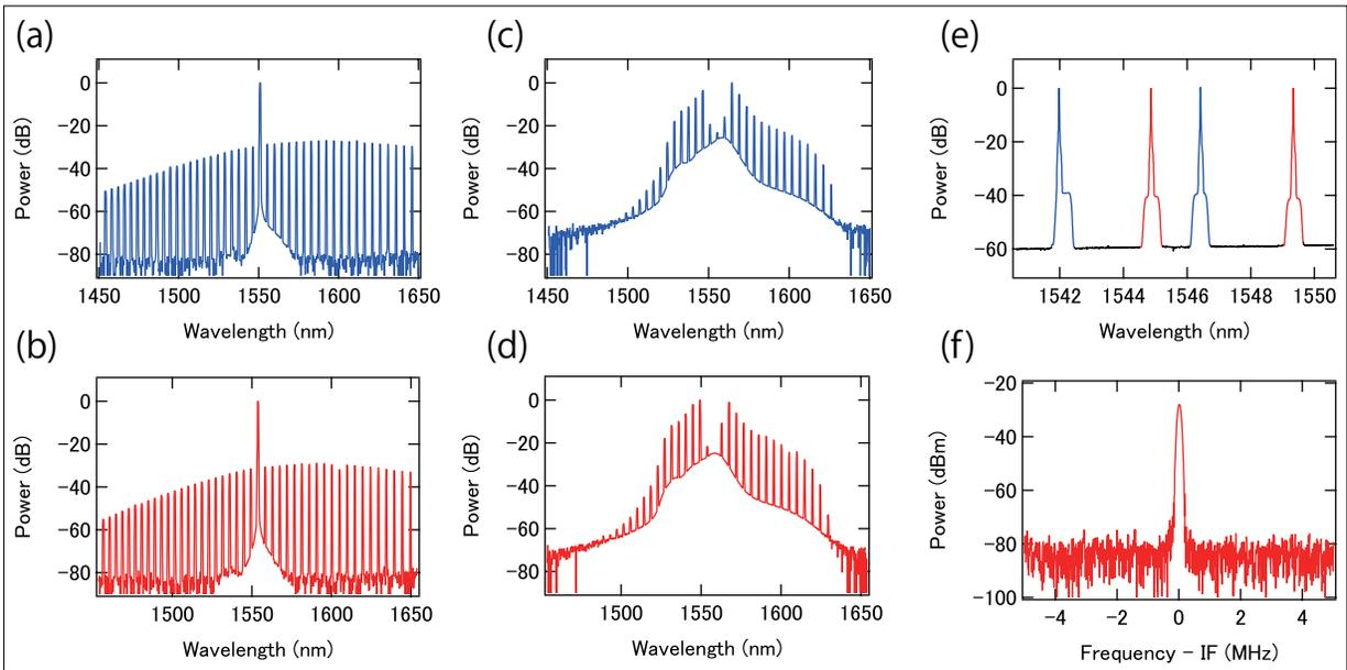
Figure 3: **Optical spectra and RF spectrum.** Optical spectra of combs 1 (a) and 2 (b) before the bandstop filter and amplified optical spectra of combs 1 (c) and 2 (d) after the bandstop filter. (e) Optical spectrum of four comb modes (blue curve from comb 1 and red curve from comb 2) used for THz waves generation. (f) RF spectrum of the microwave generated from the SBD. Resolution bandwidth (RBW) for (a) - (d) is 1 nm. RBW for (e) is 0.02 nm. RBW for (f) is 100 kHz.
