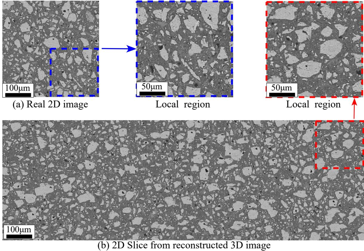
Figure 8: The generated large-size microstructural image. (a) real 2D BSE image, (b) the 2D slice from generated 3D image.
