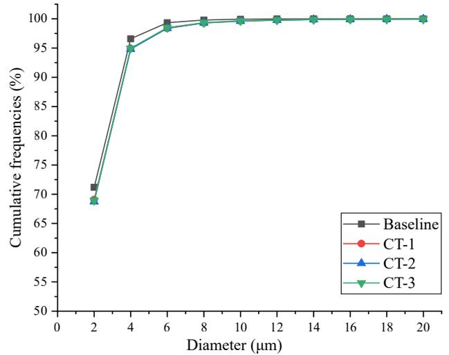
Figure 14: Pore size distribution of 3D microstructure and generated 3D microstructures. The baseline represents the real 3D microstructure, while CT-1, CT-2, and CT-3 denote three generated 3D microstructures, respectively.
