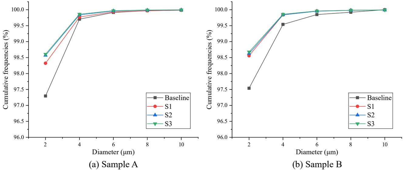
Figure 11: Pore size distribution of 2D microstructure and different-size 3D microstructures. The baseline represents the real 2D microstructure, while S1, S2, and S3 denote three generated 3D microstructures with distinct sizes, respectively.
