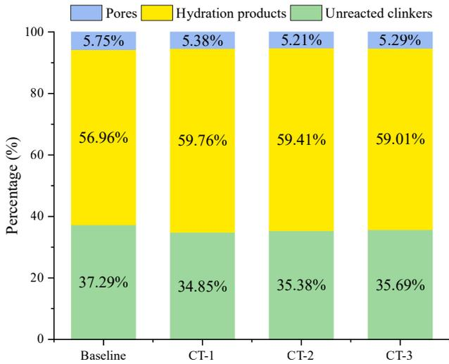
Figure 13: The various phases proportions of generated 3D microstructures and real 3D microstructure. The baseline represents the real 3D microstructure, while CT-1, CT-2, and CT-3 denote three generated 3D microstructures, respectively.
