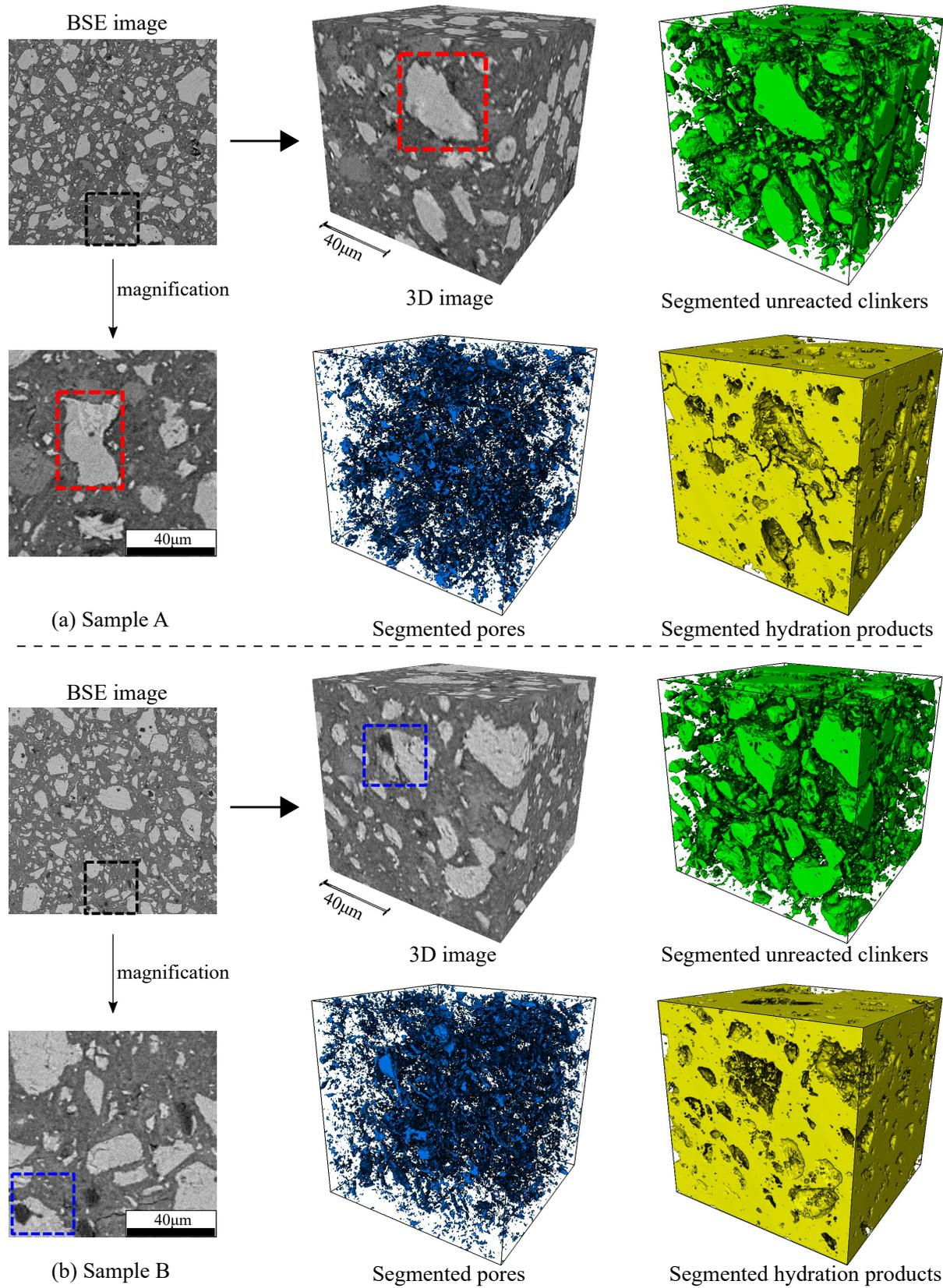
Figure 7: The generated 3D microstructural images. The left is a real BSE image, and the right are generated microstructural images. Three phases are segmented in microstructure, green denotes unreacted clinkers, blue denotes pores and yellow denotes hydration products.
