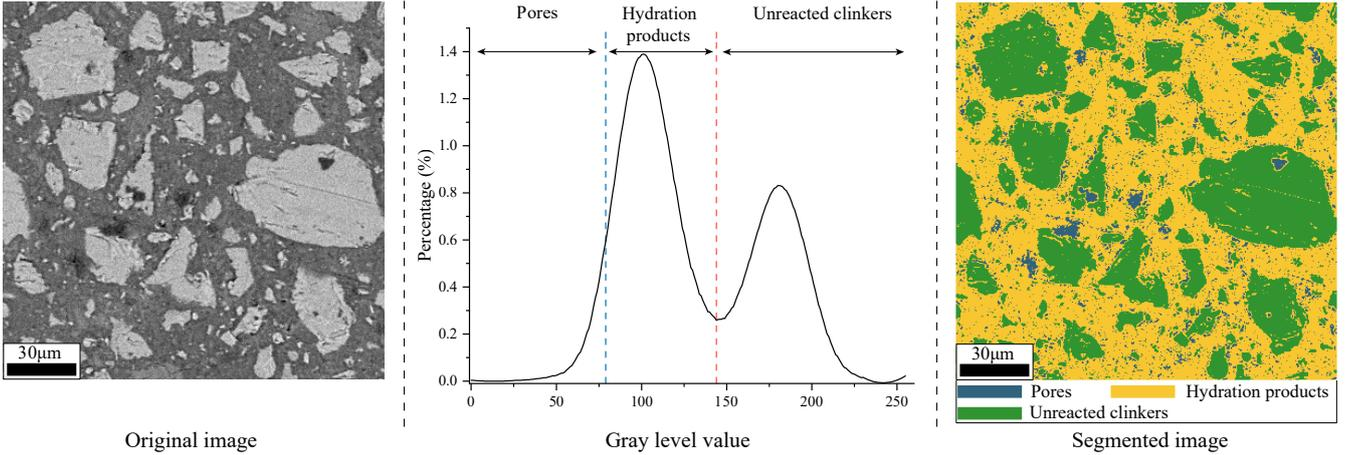
Figure 5: Phases segmentation. Pores, hydration products and unreacted clinkers are segmented based on histogram.
