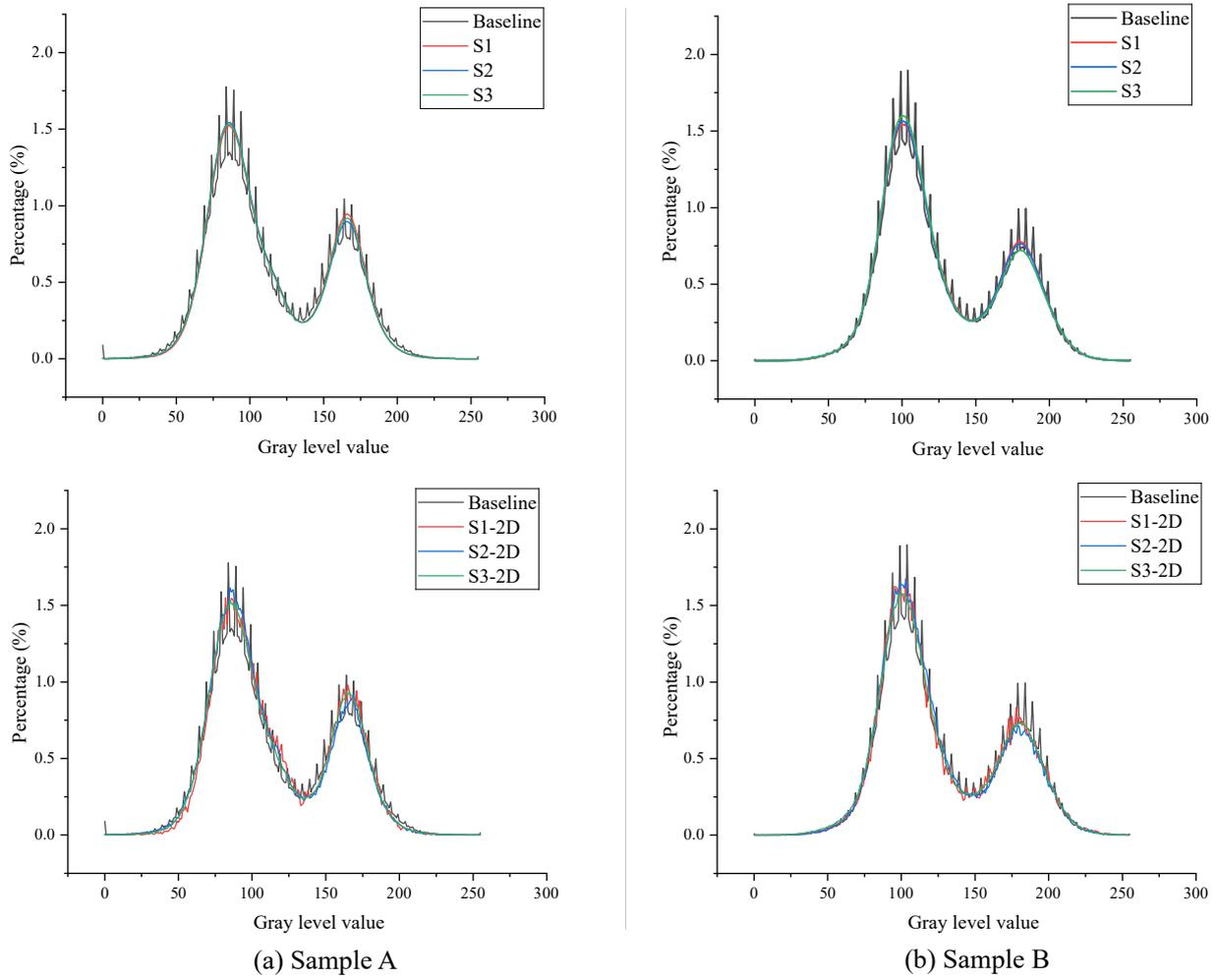
Figure 9: Gray level histograms of 2D and 3D images. The baseline represents the real 2D BSE image, while S1, S2, and S3 denote three 3D images with distinct sizes, respectively. Note that the first row displays the results of the 2D BSE image and the generated 3D image, while the second row shows the results of the 2D BSE image and the 2D slice randomly selected from the generated 3D image.
