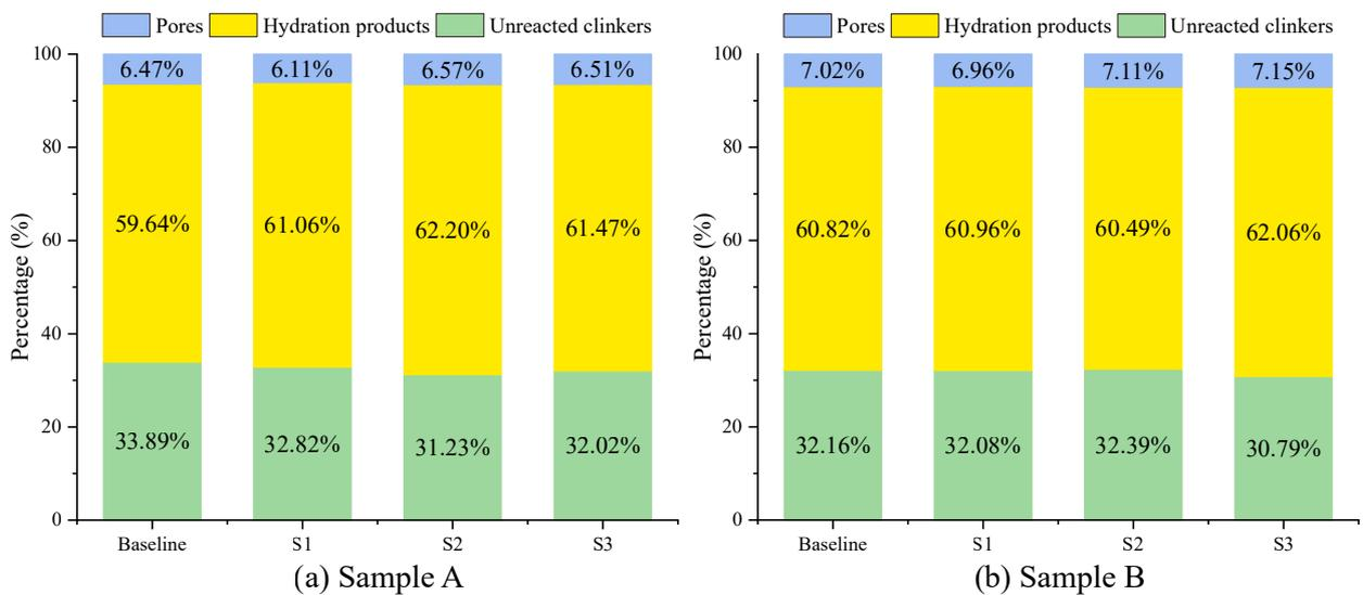
Figure 10: The various phases proportions of generated microstructures and real microstructures. The baseline represents the real 2D microstructure, while S1, S2, and S3 denote three generated 3D microstructures with distinct sizes, respectively.
