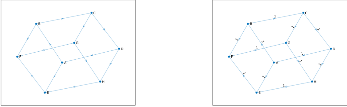
Figure 3.8: Directed graphs derived from a cube. Each corner of the cube is connected to three others by an edge. On the left no weight is assigned to any edge. On the right, all edges have a weight assigned.
