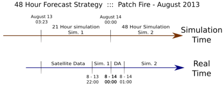
Figure 4.21: Timelines for the Patch Fire, 48-hour simulation experiment. The orange arrow indicates timings of simulations and the blue arrow indicates the progression of real-time tasks taken to produce and process the simulations in the red timeline.
