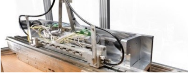
Fig. 2: Experimental coreless linear motor setup.
