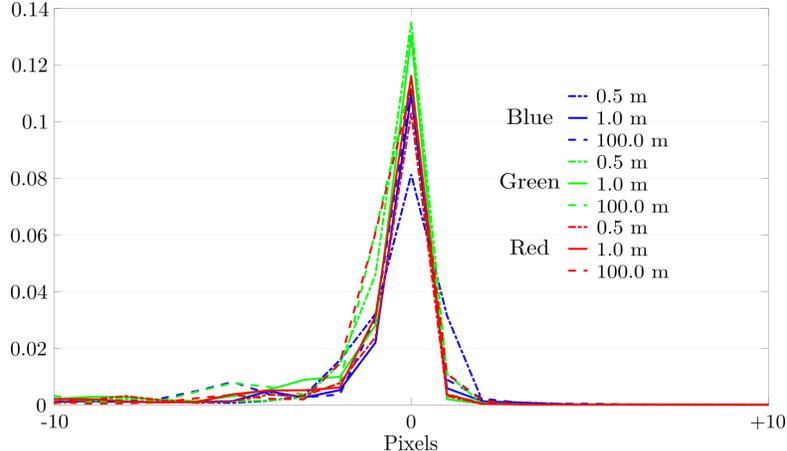
Figure 7. For the best hybrid system ( $D = 6$  mm,  $f_0 = 5$  mm), we show the cross-sections of the spectral PSFs for the three RGB channels and for the distances  $d_1$  used in Figure 5. These cross-section curves are well consolidated, what which explains a good performance of the imaging system for different distances  $d_1$  and different color channels.
