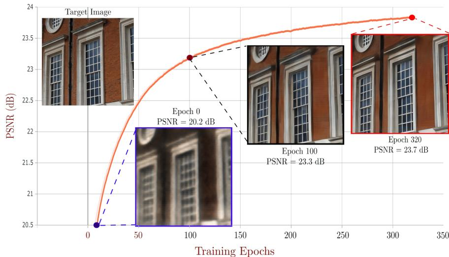
Figure 9. Performance of CNN for design of inverse imaging algorithm. The quality achieved by CNN starts from 20.5 dB and reaches 23.8 dB of PSNR for the training image set. The reconstructed images over the testing dataset are presented for three epochs 0, 100, and 320 for visualization of the training process. It could be seen that the trained network performs well for this task and the output image for epoch 320 is sharp enough.
