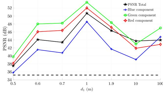
Figure 4. The spectral performance of the best-optimized hybrid system ( $D = 6mm$  and  $f_0 = 5mm$ ) is characterized by PSNRs calculated for the RGB channels as functions of  $d_1$ . All curves are above the good imaging quality line 35 dB. The curves for color components mainly follow the behavior of the total PSNR curve (black).
