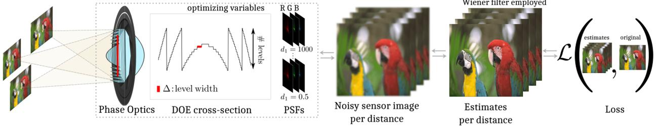
Figure 2. The optimal design framework of phase-encoded optics and image reconstruction algorithms for achromatic EDoF. The spectral PSFs are convolved with batches of RGB ground-truth images. The inverse imaging provides estimates of these images. Finally, a quality/accuracy loss  $\mathcal{L}$ , such as mean squared error with respect to the ground-truth images (or PSNR criterion), is defined on reconstructed images.
