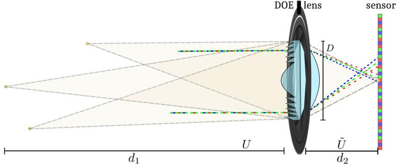
Figure 1. A light wave with a given wavelength and a curvature for a point source at a distance  $d_1$  propagates to the aperture plane containing MPM (refractive index  $n$ ) to be designed. The MPM modulates the phase of the incident wavefront. The resulting wavefront propagates through the lens to the aperture-sensor, distance  $d_2$ , via the Fresnel propagation model. The intensities of the sensor-incident wavefront define PSFs of the diffractive hybrid optical system.
