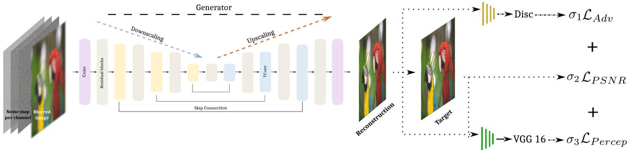
Figure 8. Inverse imaging UNet-based neural network architecture. The generator model is a U-net architecture that has seven scales with six consecutive downsampling and upsampling operations [26]. We adopt a weighted combination of PSNR between estimated and ground truth images,  $\mathcal{L}_{PSNR}$ , and perceptual losses  $\mathcal{L}_{Adv}$  and  $\mathcal{L}_{Percep}$ , with weights  $\sigma_1, \sigma_2$ , and  $\sigma_3$ .
