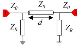
Figure S3. Transmission line circuit separated by two identical complex impedances that supports BIC and CPAs.
