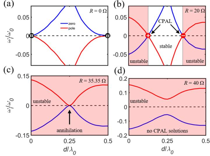
Figure S4. S-matrix pole and zero dispersion of the circuit from Fig. 4 in the main text. Solutions were found in the parameter space of  $d-\omega_i-X$  for four different  $|R|$  values (a-d). Red-shaded parts of the graphs represent the unstable regions.
