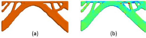
Figure 15: Final topology (a) and stress distribution (b) when the structure is subject to a spatially temperature gradient with resulting compliance and stress are as large as 4.17 and 1.98 times their initial values.
