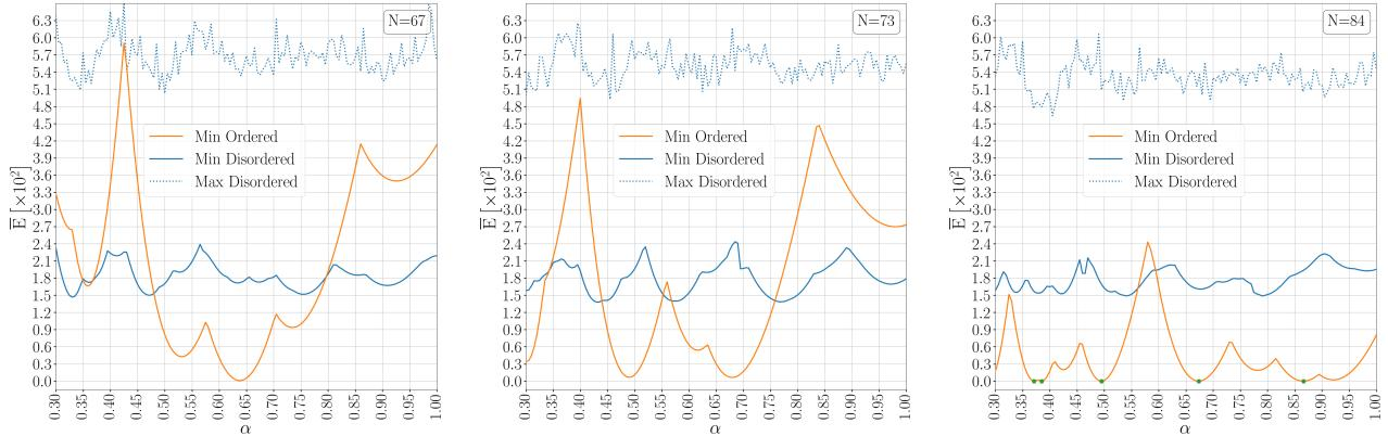
Figure 8: The minimum volumetric excess energy for ordered (orange) and disordered (blue-solid) equilibria, and maximum  $\bar{E}$  for stable disordered (blue-dotted) computational equilibria from  $\mathcal{B}(N, \alpha, 5000)$  for  $N = 67, 73, 84$  (left to right). The green dots on the  $N = 84$  minimum ordered  $\bar{E}$  curve indicate the set  $\mathcal{H}(84)$  of regular hexagonal tilings.
