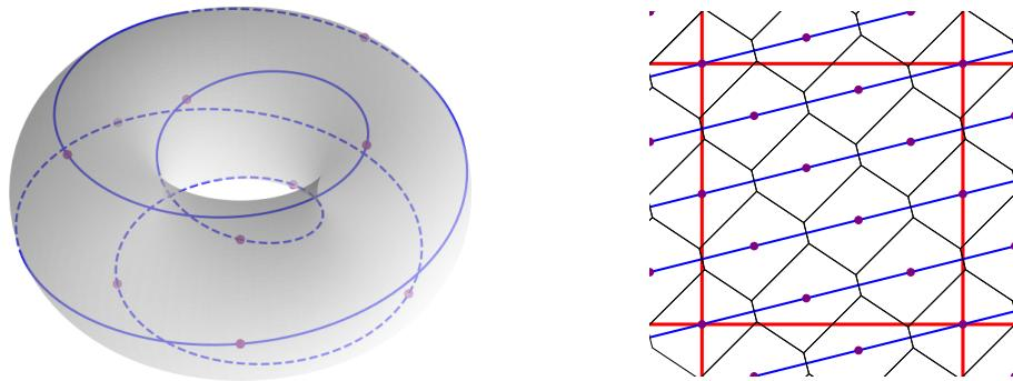
Figure 3: Construction of a single-string tessellation for  $\alpha = 1$ . (left) A closed, straight-line geodesic of the equal-radius torus  $\mathbb{T}_1$  divided into  $N = 10$  sub-units. (right) The mapping of the ten points onto  $\Omega_1$  (red lines), and the associated single-string Voronoi tessellation.
