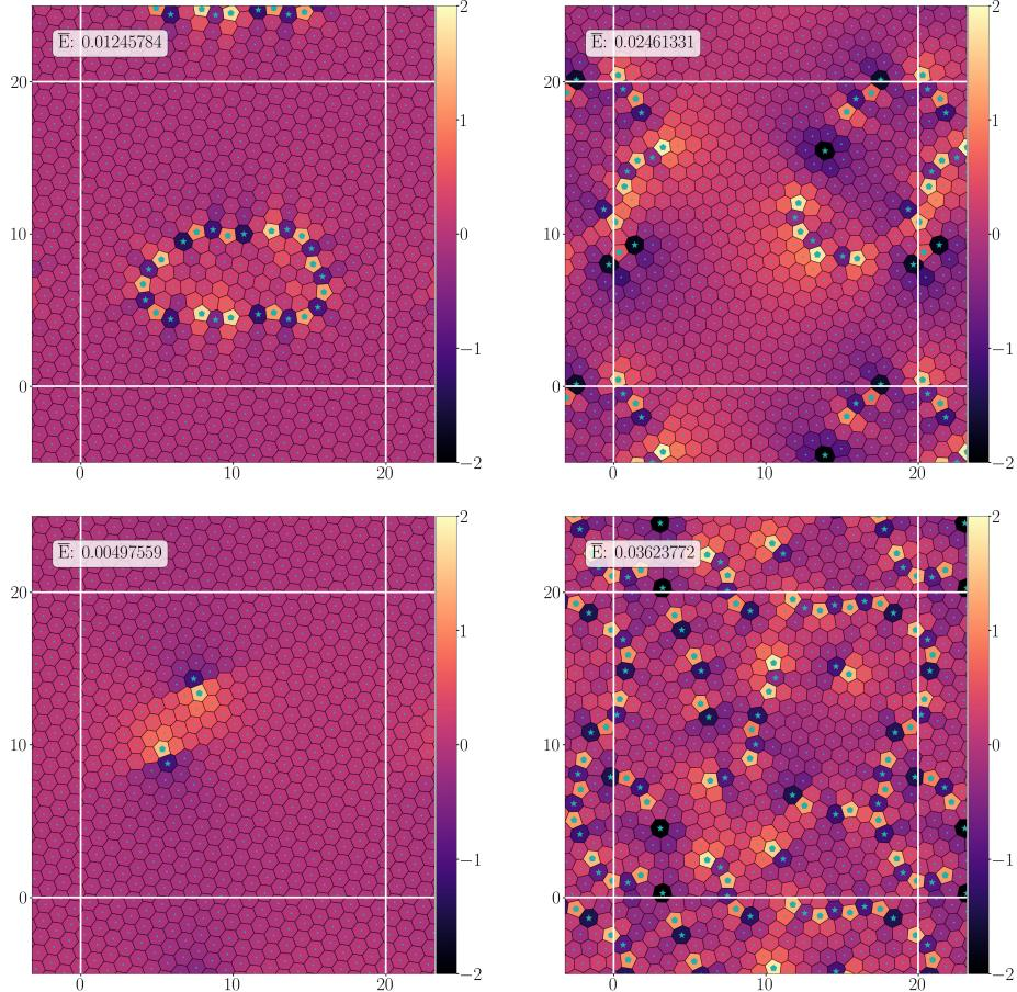
Figure 12: (top) The bin  $\mathcal{B}(400, 1, 2500)$  yielded 78 tessellations with  $D = 26$  defects. These two represent the lowest and the highest  $\bar{E}$  among this set. (bottom) The two tessellations from the bin with (left) the lowest number,  $D = 4$ , and (right) the highest number,  $D = 62$ , of defects.
