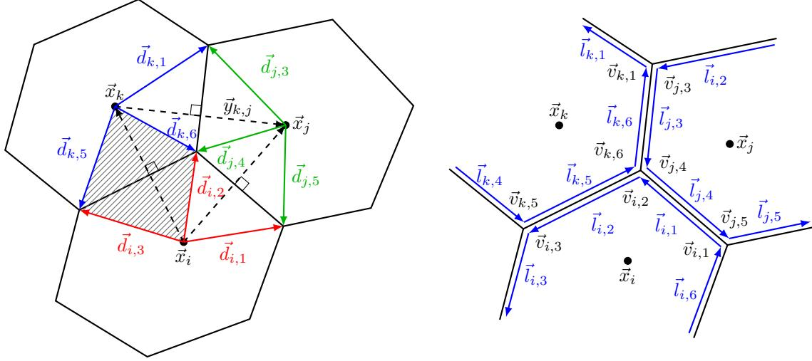
Figure 2: Sample of Voronoi cells with shared vertex  $\vec{v}$  labeled with key vectors. Relative vertex vectors  $\vec{d}$ , Voronoi edges as perpendicular bisectors, and the kite region formed between sites  $\vec{x}_i$  and  $\vec{x}_k$  are shown (left). The edge vectors  $\vec{l}$  are drawn adjacent to the edge, showing the opposing directions between neighboring sites due to the counterclockwise orientation (right).
