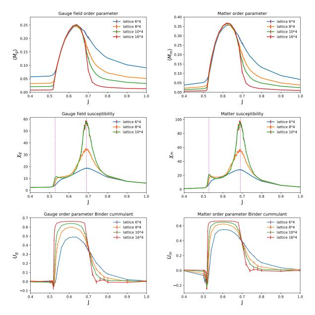
Figure 4: Vacuum expectation value (top row), susceptibility (middle row) and Binder cumulant (bottom row) for the gauge field order parameter  $M_g$  (lhs. column) and the matter order parameter  $M_m$  (rhs. column). The results are for the self-dual value  $\beta = \beta^* \equiv 1/2\pi$  and are plotted as a function of J. We compare different volumes as indicated in the legends.
