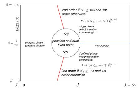
Figure 3: The conjectured phase diagram for sufficiently large  $N_f^e = N_f^m = N_f$ . The limits  $\beta \sim 0$  or  $\beta \sim +\infty$  can have a 2nd order phase transition if  $N_f \geq 183$ , as discussed in Sec. 2.5.
