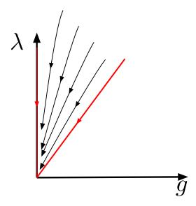
Figure 12: The RG flow is bounded by the separatrix solutions  $g = \alpha \lambda$  with  $\alpha$  given in (100) and drawn as red lines. The separatrices form a funnel which guaranties that the fixed point is reached as long as the flow is started within the funnel.
