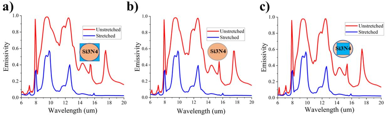
**Figure S6.** Emissivity spectra (TM polarized) of the PDMS device with a metallic substrate and (a) square  $\text{Si}_3\text{N}_4$  structures of the same size as the original cylindrical design, (b) the cylindrical structures from the main paper, and (c) square shaped structures that are slightly smaller than the original cylindrical structures.
