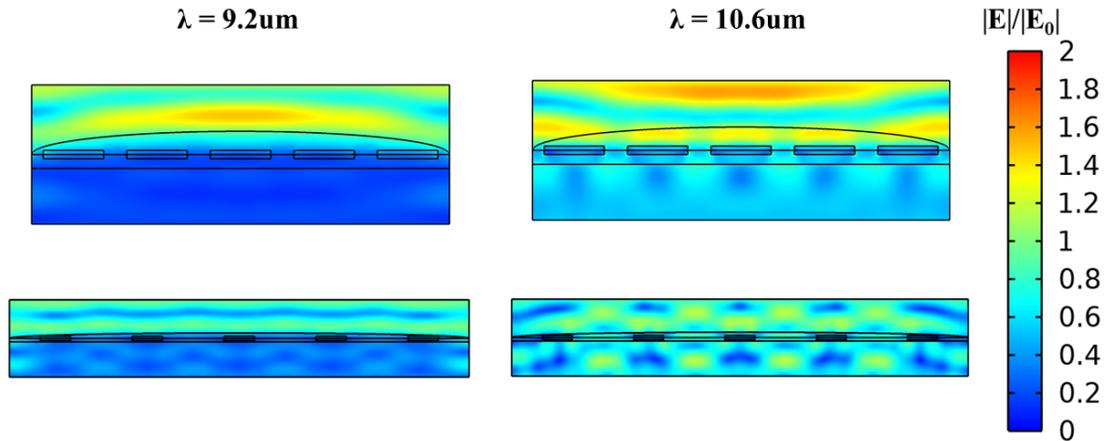
**Figure S2.** Surface plots of the electric field enhancement distributions for the rectangular  $\text{Si}_3\text{N}_4$  inclusions in the PDMS structures at the peak absorption wavelengths of PDMS ( $9.2 \mu\text{m}$ ) and  $\text{Si}_3\text{N}_4$  ( $10.6 \mu\text{m}$ ). The upper captions correspond to the unstretched structure while the lower captions to the stretched configuration.
