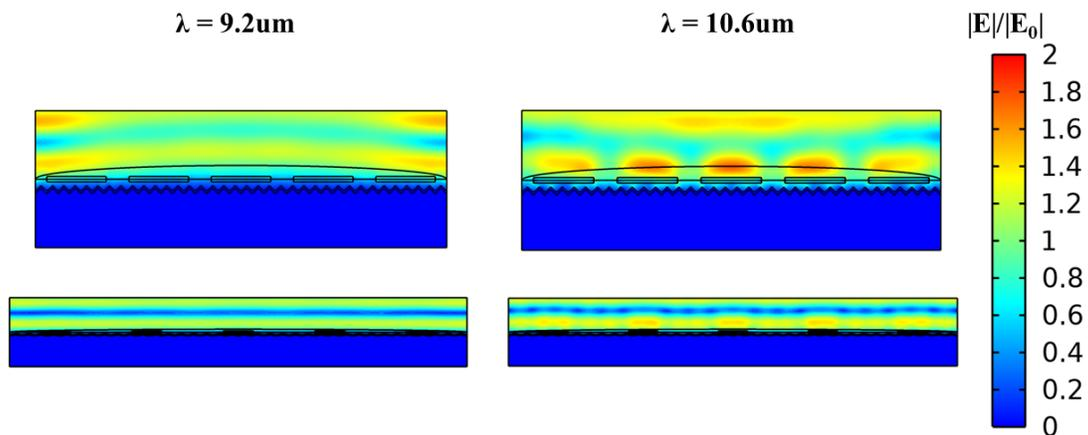
**Figure S4.** Surface plots of the electric field enhancement distributions for the rectangular  $\text{Si}_3\text{N}_4$  inclusions within the crumpled metal PDMS structures at the peak absorption wavelengths of PDMS ( $9.2 \mu\text{m}$ ) and  $\text{Si}_3\text{N}_4$  ( $10.6 \mu\text{m}$ ). The upper captions correspond to the unstretched structure while the lower captions to the stretched configuration.
