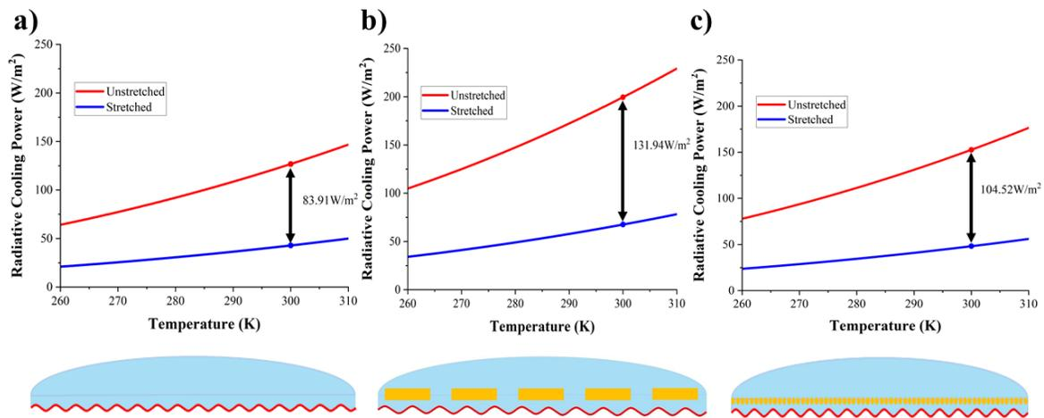
**Figure 7.** Radiated cooling power versus temperature for the PDMS over crumpled metal designs a) without  $\text{Si}_3\text{N}_4$  inclusions, b) with rectangular  $\text{Si}_3\text{N}_4$ , and c) with cylindrical  $\text{Si}_3\text{N}_4$ .
