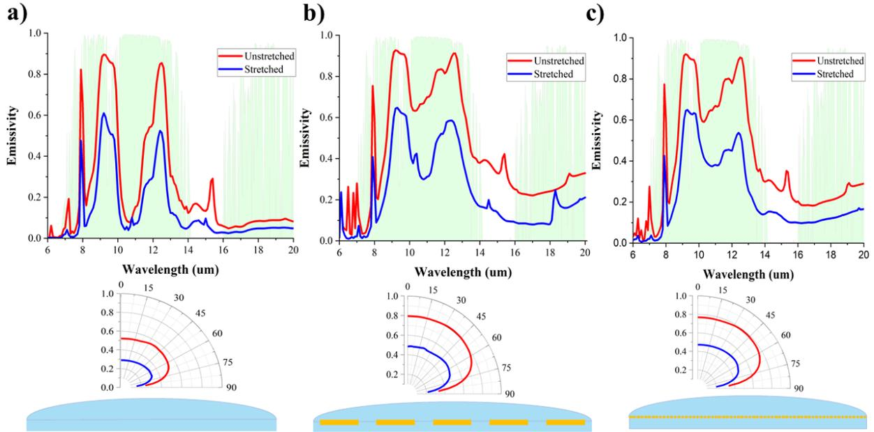
**Figure 3.** Emissivity spectra and angular emissivity of the PDMS structure a) without  $\text{Si}_3\text{N}_4$  inclusions, b) with rectangular  $\text{Si}_3\text{N}_4$ , and c) with cylindrical  $\text{Si}_3\text{N}_4$ . The green shaded area represents the atmospheric transmission window. Lower captions: angular emissivity is the average emissivity value computed over 9-13  $\mu\text{m}$  for different emission angles.
