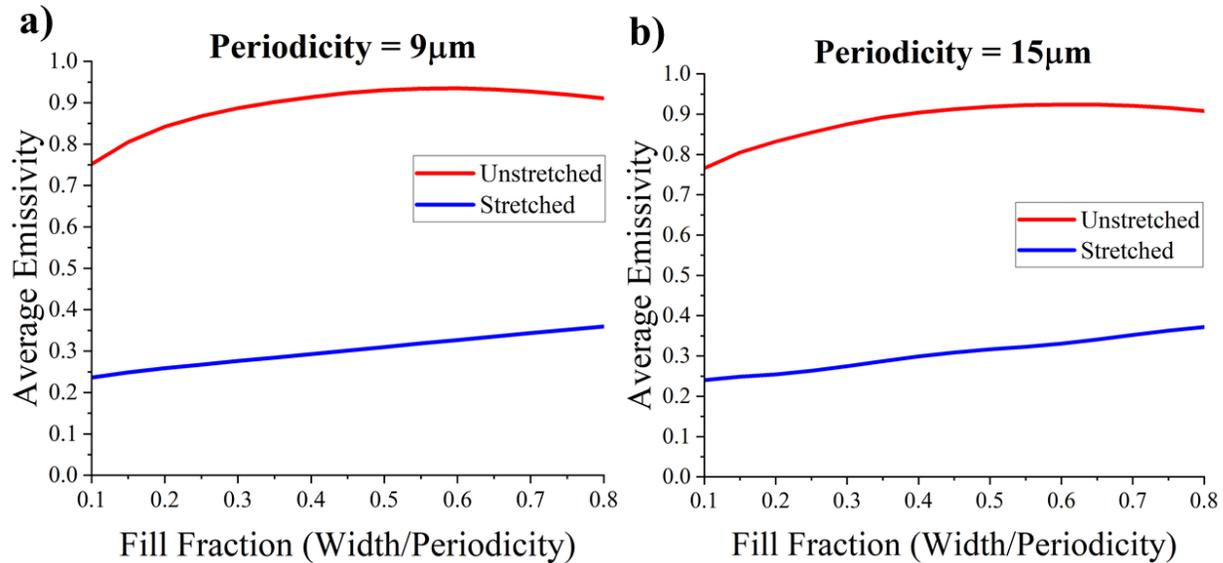
**Figure S8.** Average emissivity (TM polarized) between  $9\mu\text{m}$  and  $15\mu\text{m}$  versus the rectangular  $\text{Si}_3\text{N}_4$  fill fraction for periodicities of (a)  $9\mu\text{m}$  and (b)  $15\mu\text{m}$ .
