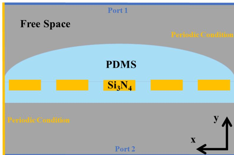
Figure S1. Schematic of the simulation domain.
