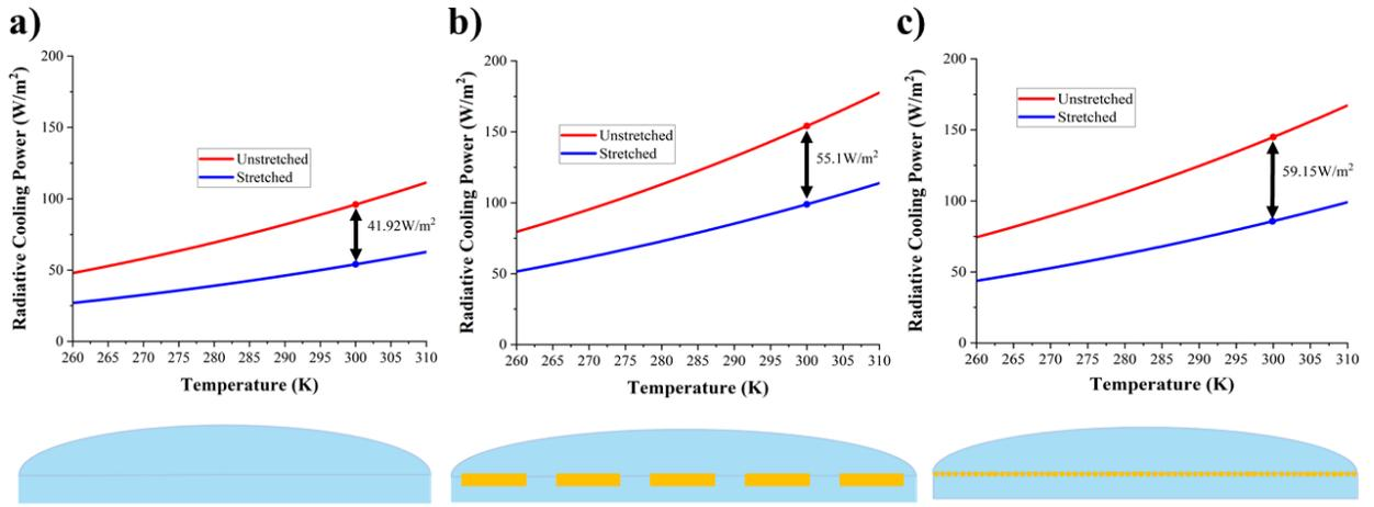
**Figure 4.** Radiated cooling power versus temperature for the PDMS structure a) without  $\text{Si}_3\text{N}_4$  inclusions, b) with rectangular  $\text{Si}_3\text{N}_4$ , and c) with cylindrical  $\text{Si}_3\text{N}_4$ .
