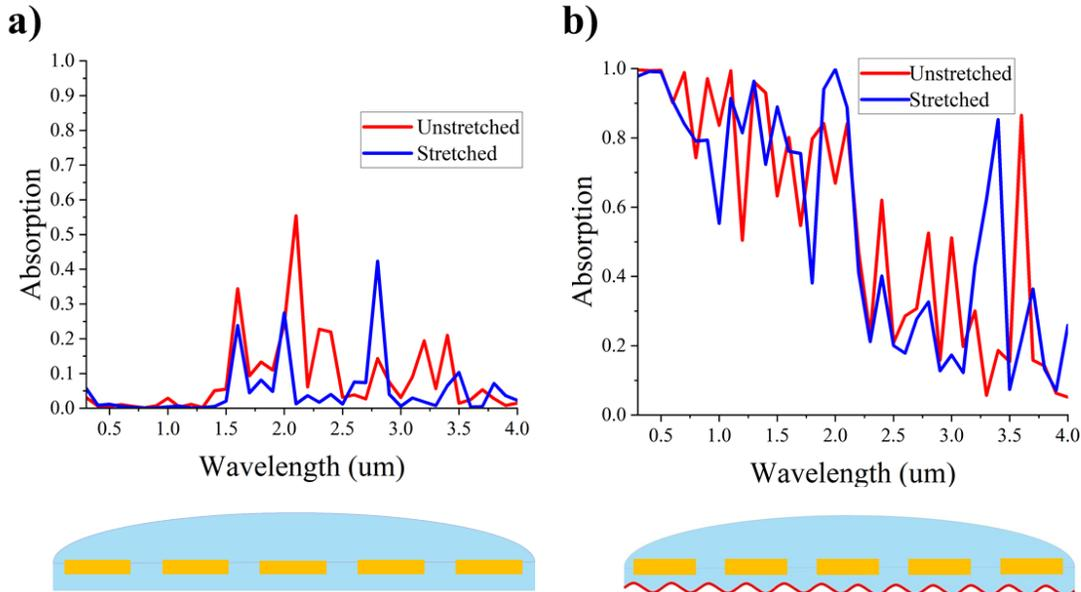
**Figure S10.** Solar absorption spectra (TM polarized) of the rectangular designs (a) without and (b) with metal substrate.
