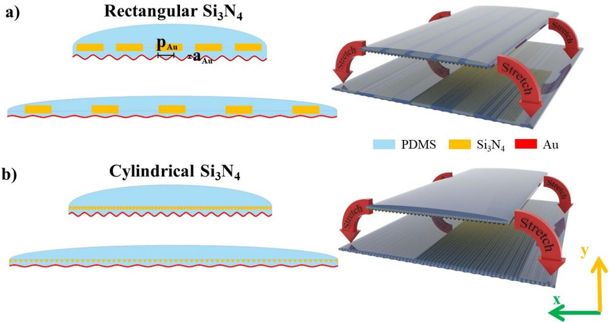
**Figure 2.** Schematic of the unit cell of two stretchable radiative cooling designs based on PDMS over crumpled metal embedded with a) rectangular and b) cylindrical  $\text{Si}_3\text{N}_4$  structures.
