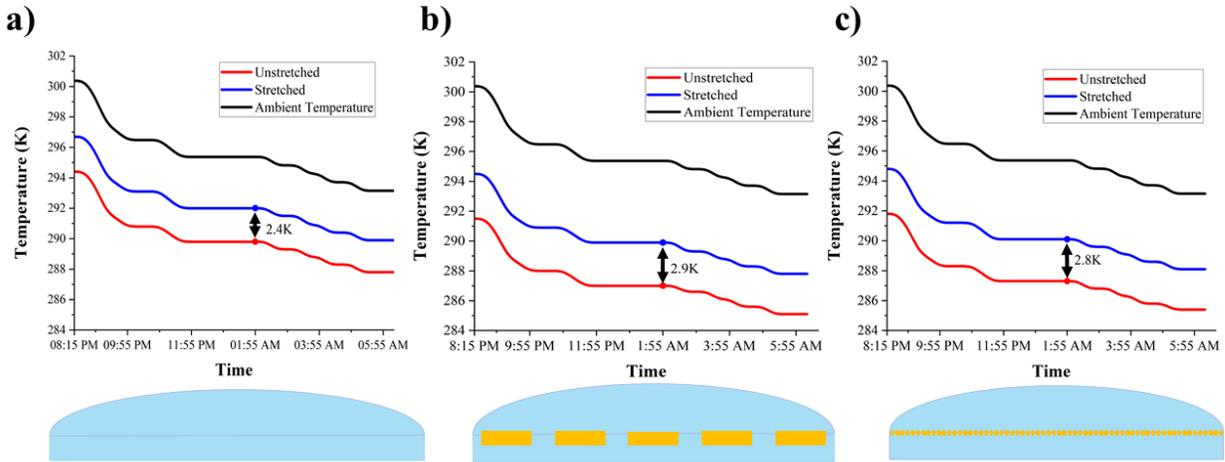
**Figure 5.** Computed hourly temperature plots for the PDMS structure a) without  $\text{Si}_3\text{N}_4$  inclusions, b) with rectangular  $\text{Si}_3\text{N}_4$ , and c) with cylindrical  $\text{Si}_3\text{N}_4$  in a terrestrial nocturnal radiative cooling scenario.
