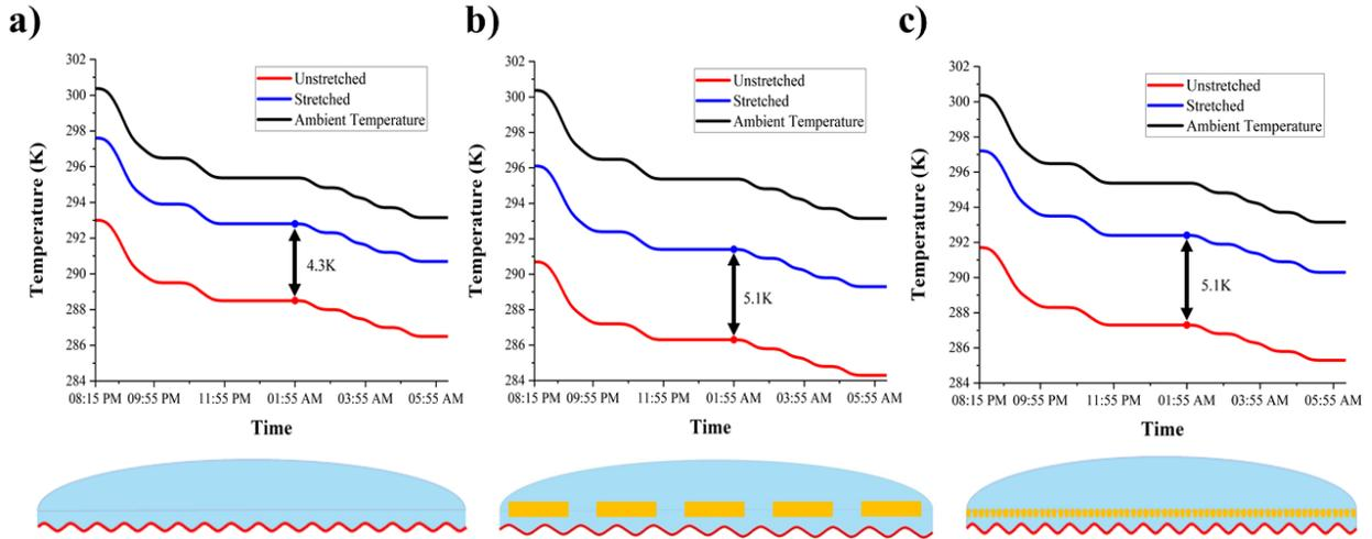
**Figure 8.** Computed hourly temperature plots of the PDMS over crumpled metal designs a) without  $\text{Si}_3\text{N}_4$  inclusions, b) with rectangular  $\text{Si}_3\text{N}_4$ , and c) with cylindrical  $\text{Si}_3\text{N}_4$  in a terrestrial nocturnal radiative cooling scenario.
