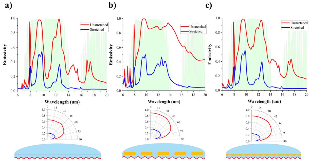
**Figure 6:** Emissivity spectra and angular emissivity of the PDMS over crumpled metal designs a) without  $\text{Si}_3\text{N}_4$  inclusions, b) with rectangular  $\text{Si}_3\text{N}_4$ , and c) with cylindrical  $\text{Si}_3\text{N}_4$ . The green shaded area represents the atmospheric transmission window. Lower captions: angular emissivity is the average value computed over 9-13  $\mu\text{m}$  for different emission angles.
