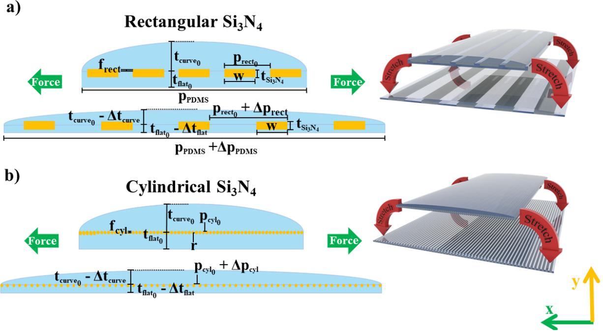
**Figure 1.** Schematic of the unit cell of two stretchable radiative cooling designs based on PDMS embedded with a) rectangular and b) cylindrical  $\text{Si}_3\text{N}_4$  structures.
