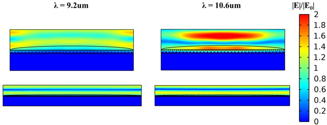
**Figure S5.** Surface plots of the electric field enhancement distributions for the cylindrical  $\text{Si}_3\text{N}_4$  inclusions within the crumpled metal PDMS structures at the peak absorption wavelengths of PDMS ( $9.2 \mu\text{m}$ ) and  $\text{Si}_3\text{N}_4$  ( $10.6 \mu\text{m}$ ). The upper captions correspond to the unstretched structure while the lower captions to the stretched configuration.
