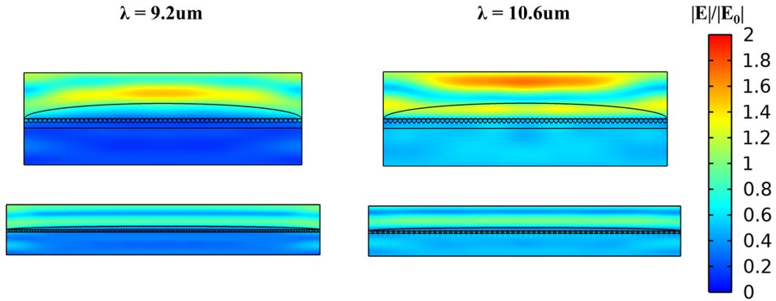
**Figure S3.** Surface plots of the electric field enhancement distributions for the cylindrical  $\text{Si}_3\text{N}_4$  inclusions in the PDMS structures at the peak absorption wavelengths of PDMS ( $9.2 \mu\text{m}$ ) and  $\text{Si}_3\text{N}_4$  ( $10.6 \mu\text{m}$ ). The upper captions correspond to the unstretched structure while the lower captions to the stretched configuration.
