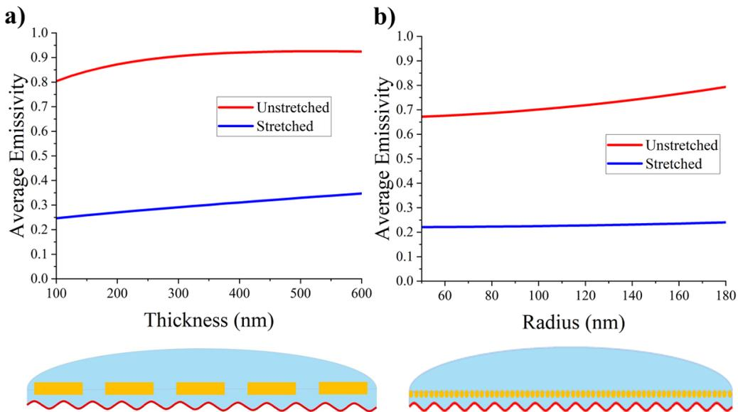
**Figure S7.** Average emissivity (TM polarized) between 9 $\mu\text{m}$  and 13 $\mu\text{m}$  versus (a) the thickness of the rectangular structures and (b) the radius of the cylindrical  $\text{Si}_3\text{N}_4$ .
