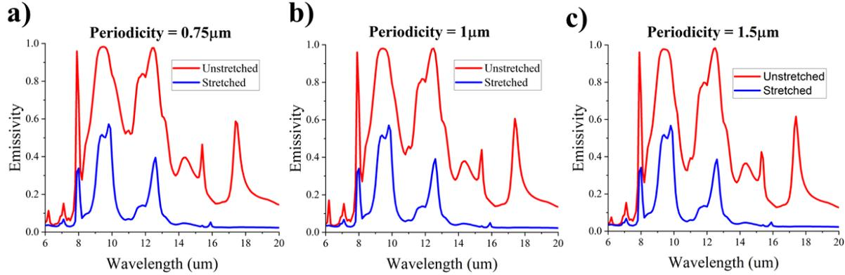
**Figure S9.** Emissivity spectra (TM polarized) of the cylindrical design for periodicities of (a) 0.75 μm, (b) 1 μm, and (c) 1.5 μm.
