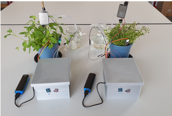
Fig. 4. Two devices of the testbed. Well visible are also the raindrop sensors and the water pumps.
