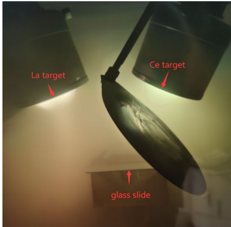
FIG. S1. Photograph of the chamber inside the magnetron sputtering equipment. The La and Ce ions were mixed in the Ar atmosphere and then deposited on a glass slide.
