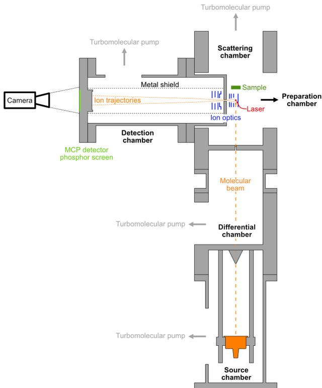
FIG. 1. Schematic diagram of the NAP-VMI apparatus.
