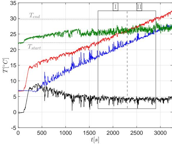
**Fig. 4.** Raw signals from thermocouples  $T_1$  (red,  $z = 0$ ) and  $T_2$  (blue,  $z = 3H/4$ ) as a function of time  $t$  for  $H = 25\text{cm}$ ,  $\Omega = 30\text{rpm}$  and  $\ell/H = 0.048$ . Also shown are the instantaneous temperature drop between the two probes (black), and room temperature (green). The solid box indicates the total measurement interval, separated by a dashed-line into two sub-intervals I and II.
