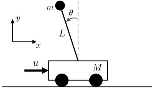
**Figure 3.** Cart-pole pendulum.
