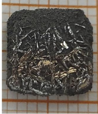
Figure 2 –Image of the surface of a Dy_{0.1}ZrTe_2 pellet after 24 hs at 1000 °C. The small reflective fragments are nucleation centers.
