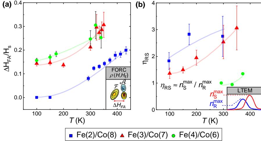
FIG. S6. **Sample-Wise  $T$ -Dependence of Stripe-to-Skyrmion Transition Characteristics.** Compiled  $T$ -dependence across the three samples of (a) FORC-measured separation of  $\mathcal{F}$  and  $\mathcal{A}$  peaks,  $\Delta H_{\mathcal{F}\mathcal{A}}$ , and (b) LTEM-measured ratio of maximal skyrmion to stripe densities,  $\eta_{RS} \equiv n_S^{\max} / n_R^{\max}$ . The trends exhibit visible sample-wise variation c.f. manuscript Fig. 4(c-d).
