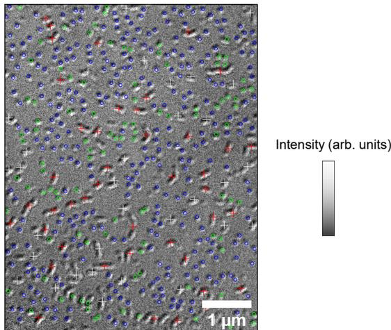
FIG. S4. **Identifying & Counting Magnetic Textures.** Representative processed LTEM image of Fe(3)/Co(7) acquired at RT,  $\mu_0 H \simeq -240$  mT, with a mixed configuration with stripes and skyrmions over a  $\sim 30 \mu\text{m}^2$  area. Textures identified as skyrmions and stripes are annotated with circles and crosses respectively. For skyrmions (stripes), blue and green (red and white) colors indicate certain and uncertain identifications of the respective magnetic textures.
