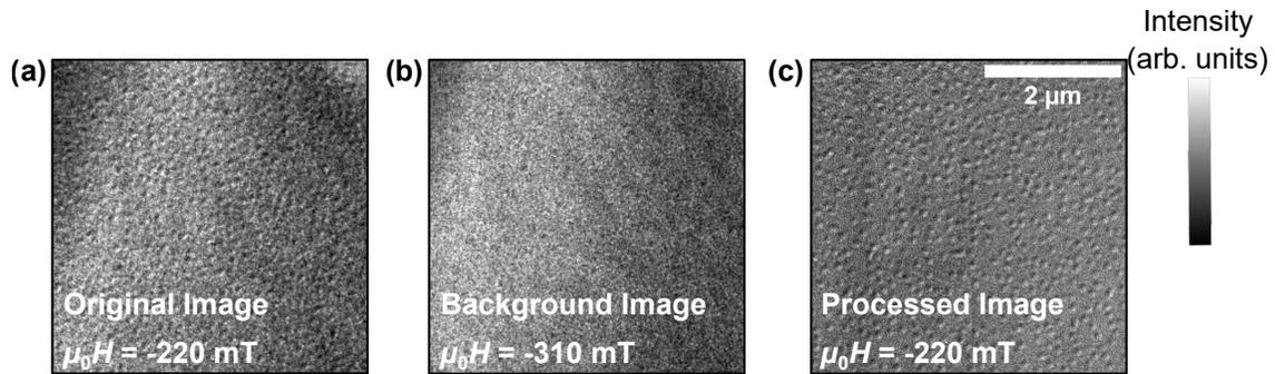
FIG. S3. **Background Removal for LTEM Images.** (a-b) As-acquired LTEM image at  $\mu_0 H \simeq -220$  mT, depicting a sparse skyrmion configuration (a), and corresponding “background” (saturated) image at  $\mu_0 H \simeq -310$  mT (b) for Fe(3)/Co(7) at RT. (c) Processed image for  $\mu_0 H \simeq -220$  mT, obtained by subtracting (b) from (a) after translating and rotating (a) to align with (b), with visibly enhanced magnetic texture contrast c.f. (a).
