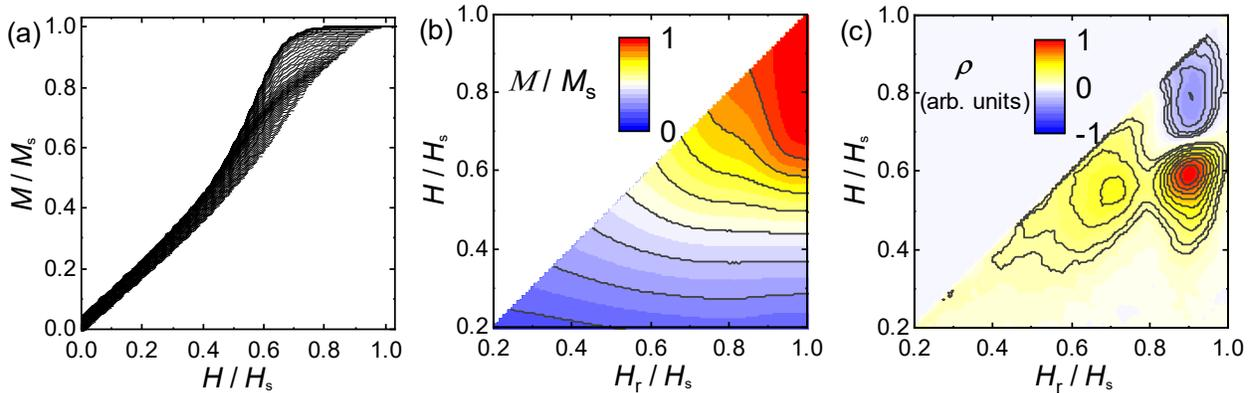
FIG. S2. **VSM and FORC measurements.** (a). Set of FORCs obtained for sample Fe(3)Co(7), with  $H_r$  and  $H$  at intervals of 2 mT. (b). Color plot of magnetisation for the FORC data in (a), projected on  $H$ ,  $H_r$  axis. (c). Color plot of  $\rho$ , the FORC irreversibility, derived from the data in (a-b).
