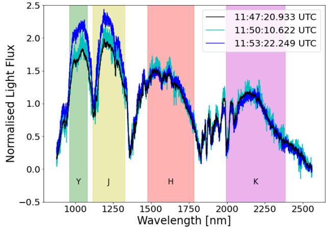
**Figure 22.** Normalized spectra obtained on the IRTF of the occultation by Ganymede on 2016-04-13. These are the spectra obtained at 11:47:20.933 (in black), 11:50:10.622 (in cyan), and 11:53:22.249 UTC (in blue). We highlight the increase in noise relative to sky fluctuations. This plot also contains the spectral region of the Y, J, H, K bands. For more information, see text.
