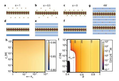
Fig. 7 | Changes in hydration structure with ion complexation. (a-c) Ion configurations at different values of  $\alpha$ . (d-f) Hydration profiles corresponding to different values of  $\alpha$ . (g) Conceptual representation of a 4W hydrate. (h) Fraction of unbound cations as a function of electrolyte concentration and water activity. (i) Hydration free energy in the high mineral volume fraction regime.
