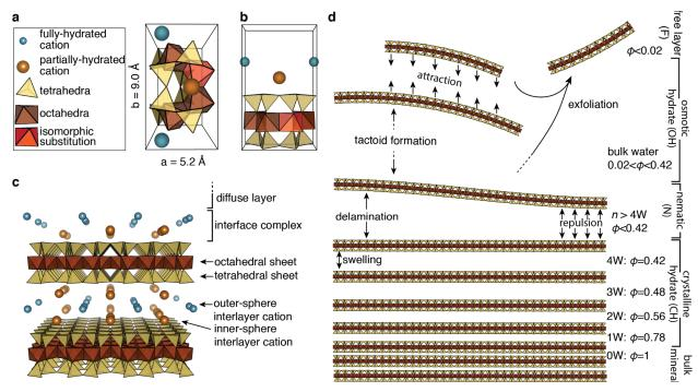
Fig 1 | Hierarchical clay mineral structures of a dioctahedral TOT layer. (a) Fundamental units of clay structures, arranged into unit cell viewed along stacking direction. (b) View of unit cell along plane of layer. (c) Ion configurations at interface with bulk solution and between layers (water molecules not shown for clarity). (d) Common structural motifs observed with varying water activity (varying mineral volume fraction).
