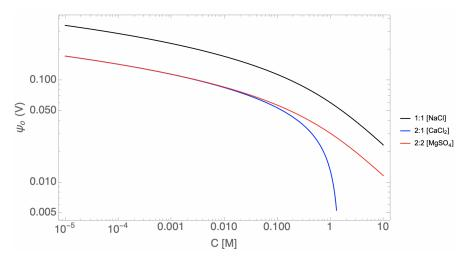
Fig S1 | Interface potential as a function of electrolyte concentration given by the Graheme equation (Eq. 2) for 1:1, 2:1 and 2:2 electrolytes.
