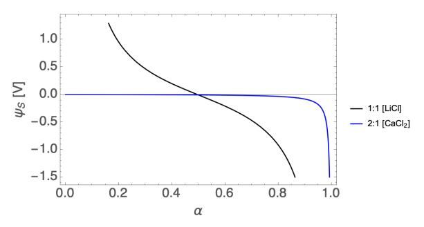
Fig S6 | Stern potential drop for LiCl and CaCl<sub>2</sub> electrolytes as a function of surface binding.
