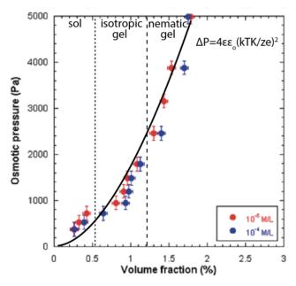
Fig S5 | Osmotic pressure of Na-Swy-2 as a function of mineral volume fraction, modified from[30] with fit to Eq. 11.
