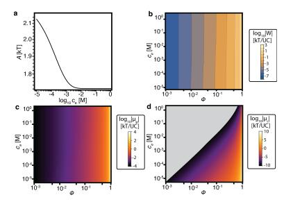
Fig 5 | van der Waals free energy and chemical potential. Variation of the Hamaker coefficient A with electrolyte concentration. (b) Magnitude of  $W_{vdW_2}$  which is minimally impacted by electrolyte concentration. (b). (c, d) van der Waals chemical potentials of electrolyte and clay.
