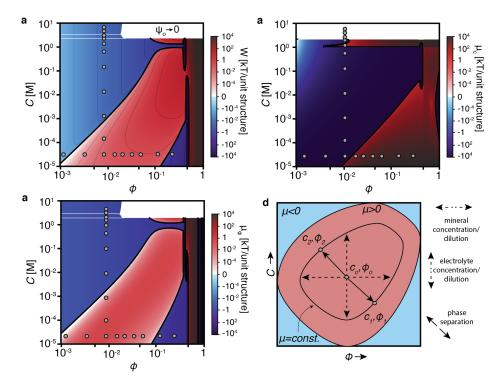
Fig. 10 | (a) FES of Ca-Mt. (b) Electrolyte chemical potential for Ca-Mt. (c) Mineral chemical potential for Ca-Mt. (d) Schematic of phase separation, showing changes in both c, and  $\varphi$  to states with equivalent chemical potentials.
