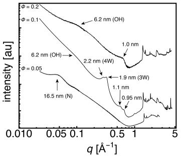
Fig S4 | 4W hydrate coexisting with 3W hydrate, which each exhibit different interfacial binding configurations as evidenced by different harmonic peaks
