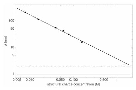
Fig S3 | Relationship between Mt charge concentration and *N* interlayer spacing in the absence of added electrolyte.
