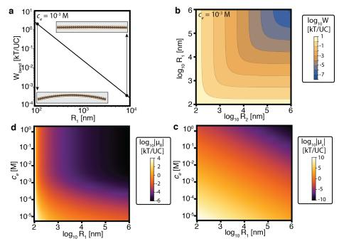
Fig 4 | Bending free energy. (a) Magnitude of  $W_{bend}$  for positive and negative curvature. (b) Variation of  $W_{bend}$  with the two principal curvature components. (c, d) bending chemical potentials of electrolyte and clay.
