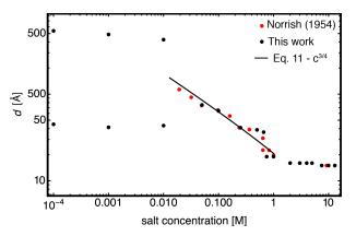
Fig 6 | Interlayer spacing of Li-Mt as a function of added LiCl concentration. Data from Fig. 2k is compared with classical observations by Norrish[7].
