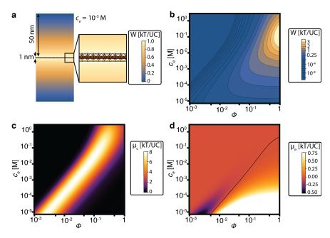
Fig 3 | Osmotic free energy and chemical potentials. (a) Magnitude of  $W_{osmotic}$  experienced by a Mt layer at a distance D from a (hypothetical) neighboring layer. (b) Variation of  $W_{osmotic}$  with clay and electrolyte concentration. (c, d) Chemical potentials of clay and electrolyte.
