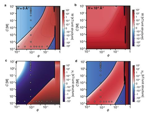
Fig. 8 | Smectite free energy and chemical potential surfaces, with experimental data points shown in gray. (a) Total free energy in the absence of curvature. (b) Total free energy in the presence of curvature. (c) Electrolyte chemical potential. (d) mineral chemical potential.
