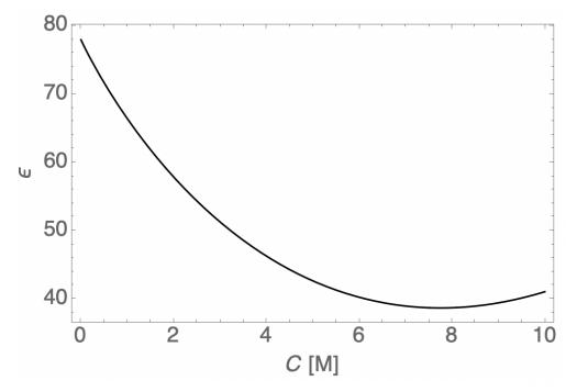
Fig S8 | Dielectric constant of bulk NaCl solution as a function of electrolyte concentration.
