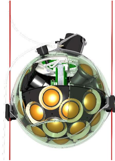
Figure 4 Rendition of an optical module as mounted with bollards attached to the supporting ropes of a detection unit. For illustration purposes, several parts are cut out. The breakout-box which connects to the backbone cable of the detection unit (see section 3.4) is attached to the top of the module.
