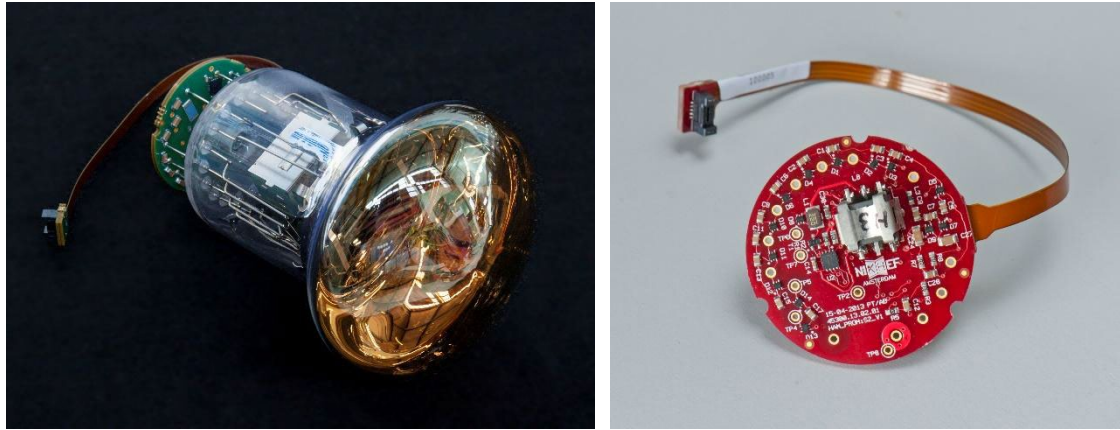
Figure 7 (Left) A Hamamatsu R12199-02 photomultiplier tube with base attached. (Right) A photomultiplier base.
