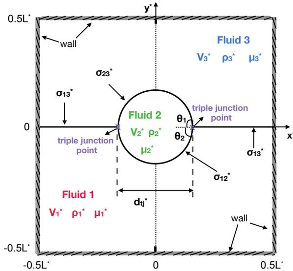
Figure 2: Geometry and initial setup of the spreading of a droplet between two stratified fluids problem.
