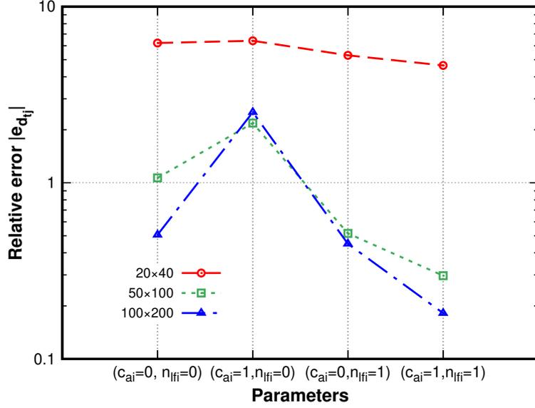
Figure 5: The relative error of the drop’s length at equilibrium  $e_{d_{tj}}$  between theory and numerical predictions for various combinations of the parameters  $C_{a_i}$  and  $n_{lfi}$  and three computational meshes consisting of  $20 \times 40$ ,  $50 \times 100$ , and  $100 \times 200$  control volumes.  $We_{p,1} = We_{p,2} = We_{p,3} = 60$ , and the density and viscosity ratios are  $\rho_i = 1$  and  $\mu_i = 1$ , respectively.
