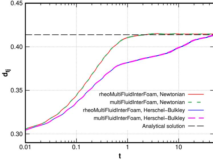
Figure 12: Time evolution of the interfaces of a floating lens with a non-Newtonian lower fluid for  $Re = 1$  and  $We_{p,1} = We_{p,2} = We_{p,3} = 60$ . The results are obtained by using the `multiFluidInterFoam` and `rheoMultiFluidInterFoam` solvers together with the bounded bi-viscosity Herschel–Bulkley model,  $Bn = \tau_{0,1}^* R_d^* / (k_1^* U^*) = 0.15$ ,  $\mu_{0,1}^* / k_1^* = 100$ , and  $n_1 = 1$ .
