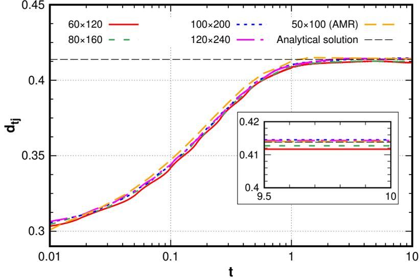
Figure 6: Time evolution of the interfaces of a floating lens for  $We_{p,1} = We_{p,2} = We_{p,3} = 60$  for various fixed uniform computational meshes  $60 \times 120$ ,  $80 \times 160$ ,  $100 \times 200$ ,  $120 \times 240$ , and an adaptive mesh of  $50 \times 100$  with a minimum non-dimensional grid spacing of  $1/200$ . The density and viscosity ratios are  $\rho_i = 1$  and  $\mu_i = 1$ , respectively.
