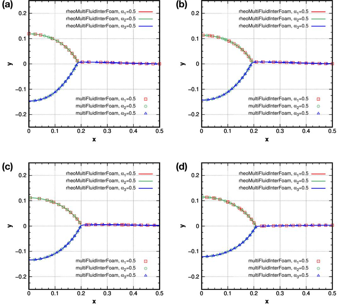
Figure 13: Shape of a floating lens with a non-Newtonian lower fluid for  $Re = 1$  and  $We_{p,1} = We_{p,2} = We_{p,3} = 60$  at non-dimensional times  $t = 1$  (a),  $t = 10$  (b),  $t = 25$  (c), and  $t = 50$  (d). The results are obtained by using the `multiFluidInterFoam` and `rheoMultiFluidInterFoam` solvers together with the bounded bi-viscosity Herschel–Bulkley model,  $Bn = \tau_{0,1}^* R_d^* / (k_1^* U^*) = 0.15$ ,  $\mu_{0,1}^* / k_1^* = 100$ , and  $n_1 = 1$ .
