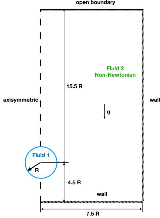
Figure 9: Geometry and configuration of a bubble rising in a viscoplastic fluid.
