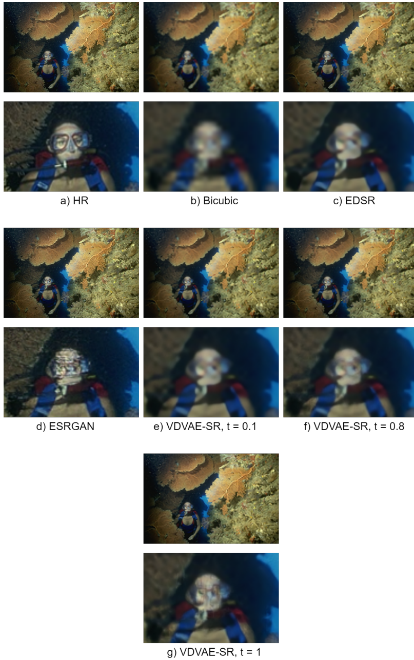
Fig. 13. SR output comparison between multiple models for picture 156065 of the BSD100 dataset.
