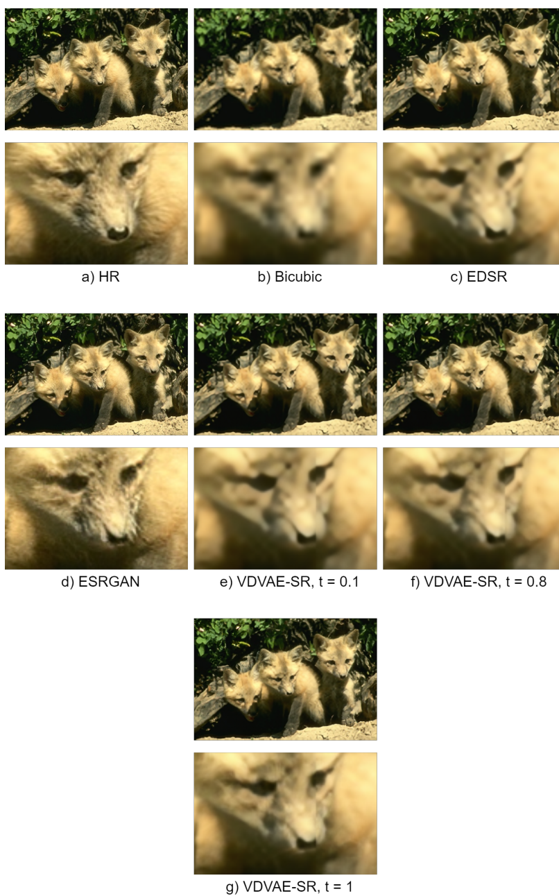
Fig. 16. SR output comparison between multiple models for picture 159008 of the BSD100 dataset.
