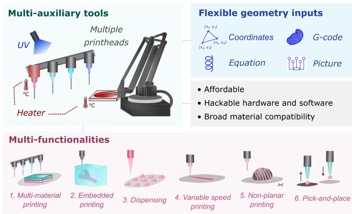
Figure 1. Features of Printer.HM, which consists of multi-auxiliary tools as hardware, flexible geometry inputs as software, leading to multi-functionalities in one-platform.
