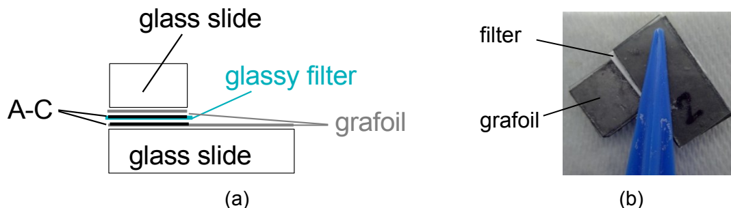
Figure 2. (a) A cross section of sample with grafoil coated active-carbon (A-C) electrodes, and (b) a picture of the cover area ca, 12.7x12.7 mm 2 .
