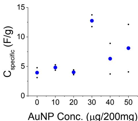
Figure 9. Specific capacitance values derived from C-V data for PVA binder and 1 M NaCl electrolyte. The black dots are the results from two sets of experiments; the blue dots are averages of these two experiments. The concentration of AuNP in  $\mu\text{g}$  is referenced to 200 mg of A-C in the batch. Large fluctuations above 40  $\mu\text{g}$  per 200 mg of A-C are result of charged AuNPs packing.
