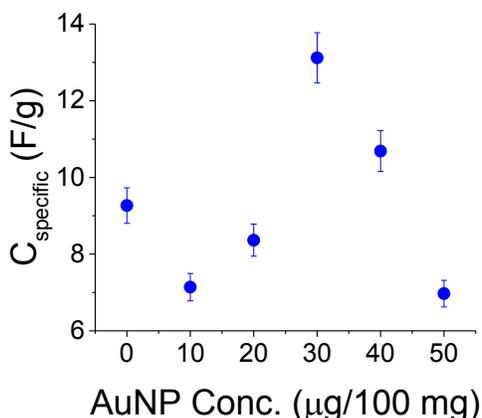
Figure 8. Specific capacitance values derived from C-V data for CAB binder and 1 M NaCl electrolyte. Similar trend is obtained with C-D data. The concentration of AuNP in  $\mu\text{g}$  is referenced to 100 mg of A-C in the batch.
