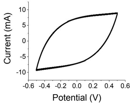
Figure 12: 125 C-V scans for the 30  $\mu\text{g}$  of AuNPs per 200 mg of A-C sample in 1 M  $\text{Na}_2\text{SO}_4$  at a rate of 50 mV/s exhibited <2% change between the first and last scan; .
