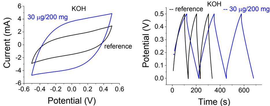
Figure 13: Replacing the 1 M  $\text{Na}_2\text{SO}_4$  electrolyte by 1 M KOH while retaining the same electrodes. (a) C-V traces at a scan rate of 20 mV/s help assess the enhancement factor of the specific capacitance as  $\sim 3$ . (b) C-D traces at an applied current of  $I_0=1$  mA (charge density,  $J_0=0.62$  mA/cm<sup>2</sup>) help assess the enhancement factor of the specific capacitance as  $\sim 4.5$ .
