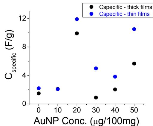
Figure 7. Specific capacitance,  $C_{\text{specific}}$  in units of F/g from C-V data for thick and thin films with a CAB binder. The concentration of AuNPs is referenced to the amount of A-C in the slurry. The  $C_{\text{specific}}$  value for  $10 \text{ }\mu\text{g}$  per 100 mg of A-C is identical for both films. The electrolyte was 1 M of  $\text{Na}_2\text{SO}_4$ .
