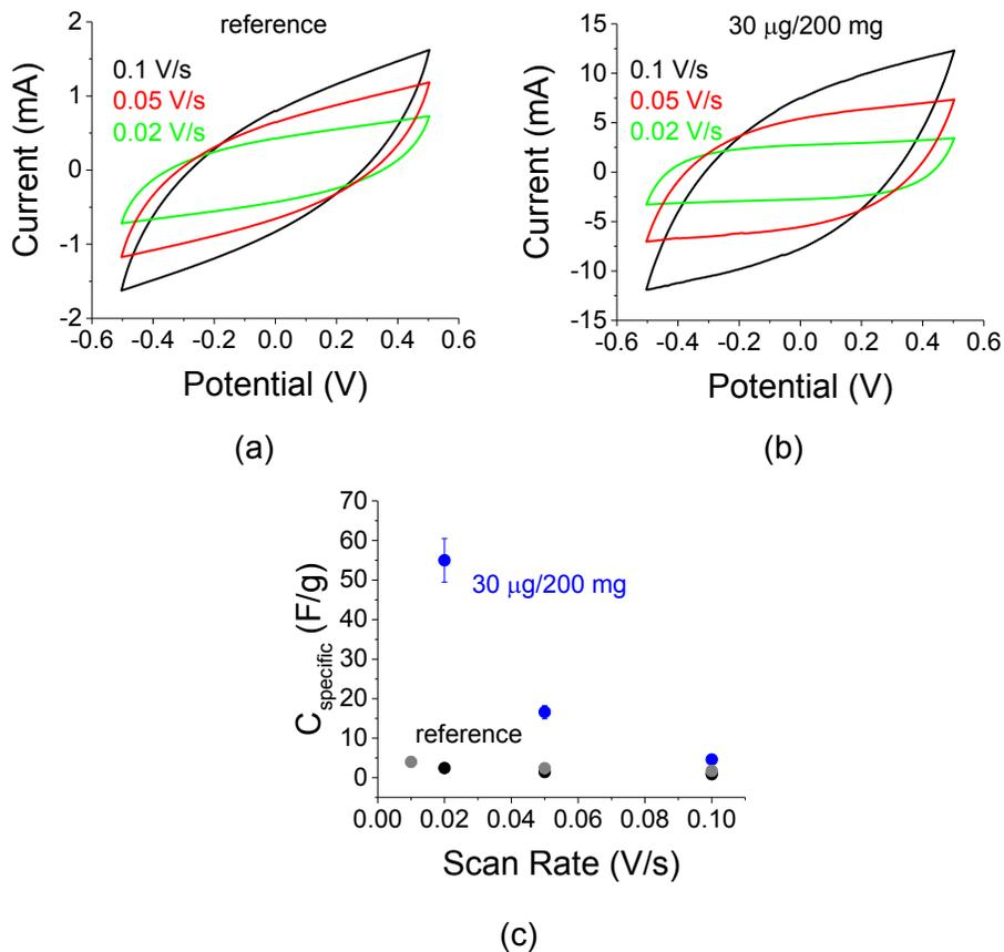
Figure 11: C-V data as a function of various scan rates for (a) reference sample (no AuNPs) and (b) with 30  $\mu\text{g}$  of AuNPs per 200 mg of A-C in a 1 M  $\text{Na}_2\text{SO}_4$  electrolyte. (c) The gravitonic specific capacitance as a function of the scan rate. The experiment for the reference sample was repeated twice (the gray and black dots).
