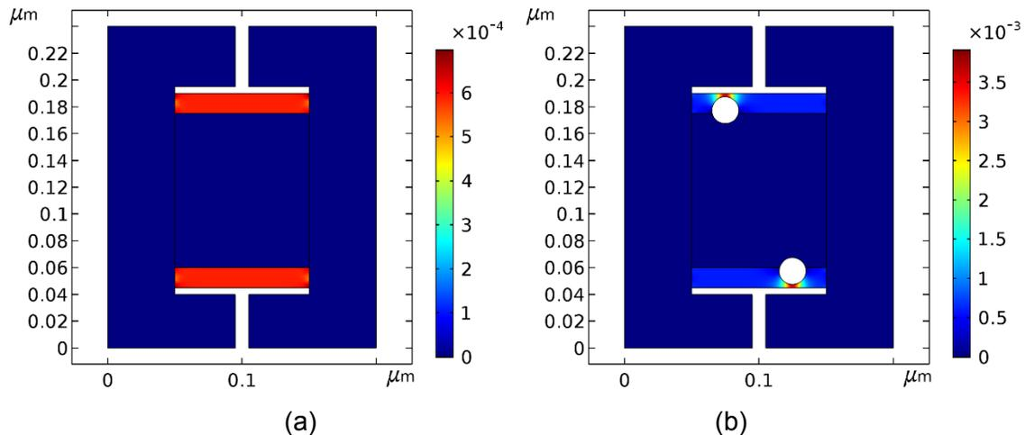
Figure 15. The absolute value of polarization is stronger near the colloids. The thermal legend is in units of  $C/m^3$ .
