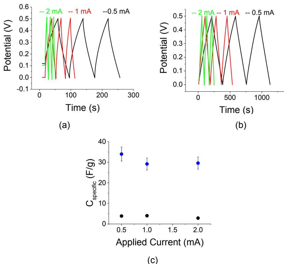
Figure 10: C-D data as a function of various current levels:  $I_0=0.5, 1$  and  $2$  mA ( $J_0=0.31, 0.62$  and  $1.24$  mA/cm<sup>2</sup>, respectively) for: (a) reference sample (no AuNPs) and (b) with  $30$  μg of AuNPs per  $200$  mg of A-C. (c) The gravitonic specific capacitance as a function of the applied current for the AuNPs sample (blue dots) and the reference (black dots).
