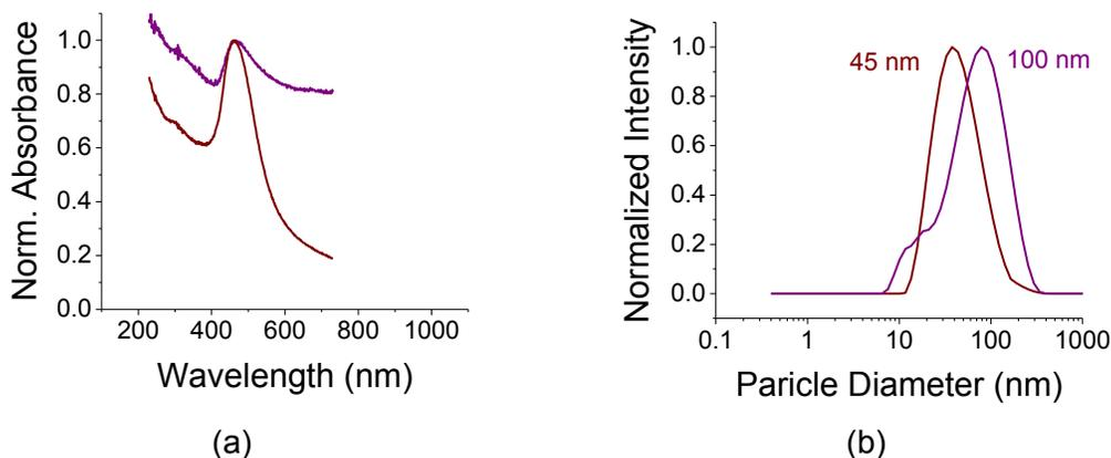
Figure. 1. (a) Absorbance (normalized such that the peak equals unity) for ligand-coated, small size (wine color) and aggregates (purple color) of AuNPs. Both were suspended in water. The plasmonic absorption is clearly seen; the aggregate peak is a bit red-shifted and broader compared to small particles' peak. The increase in absorption towards the UV spectrum is attributed to an increased scattering. (b) The corresponding DLS data show the two particle sizes used in the experiments.
