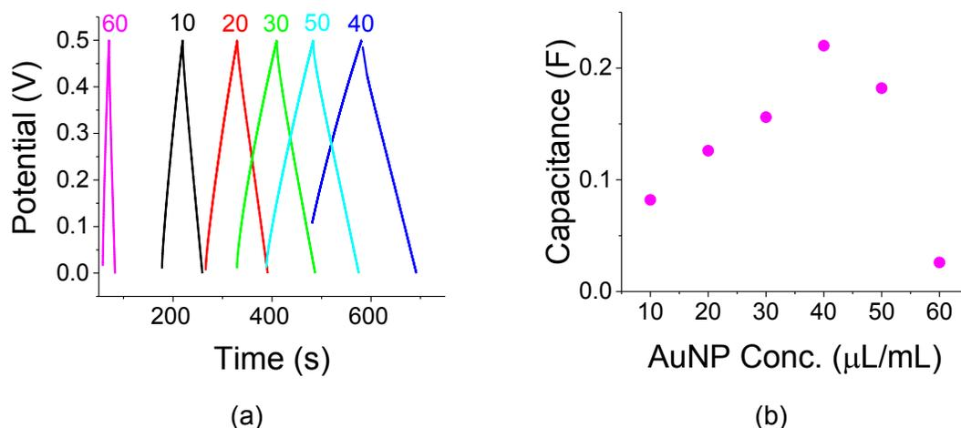
Figure 5. (a) C-D plots for various AuNPs concentration (in  $\mu\text{L}$  per 1 mL of solvent). Current used was  $I_0=1$  mA (charge density,  $J_0=0.62$  mA/cm<sup>2</sup>). (b) Capacitance as a function of AuNPs concentration exhibits a peak at 40  $\mu\text{L}/\text{mL}$ . The electrolyte was 1 M of Na<sub>2</sub>SO<sub>4</sub>.
