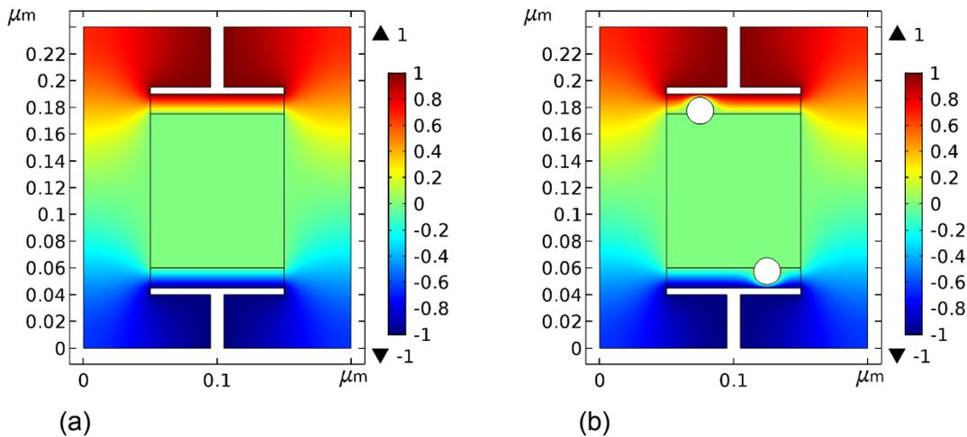
Figure 14. Potential distribution for  $V_{in}=1$  V. The neutral region indeed has a constant potential (zero in this case) and the presence of the metallic colloid alters the potential lines. (a) No colloid. (b) With 10 nm colloids. The thermal legend is in units of Volts.
