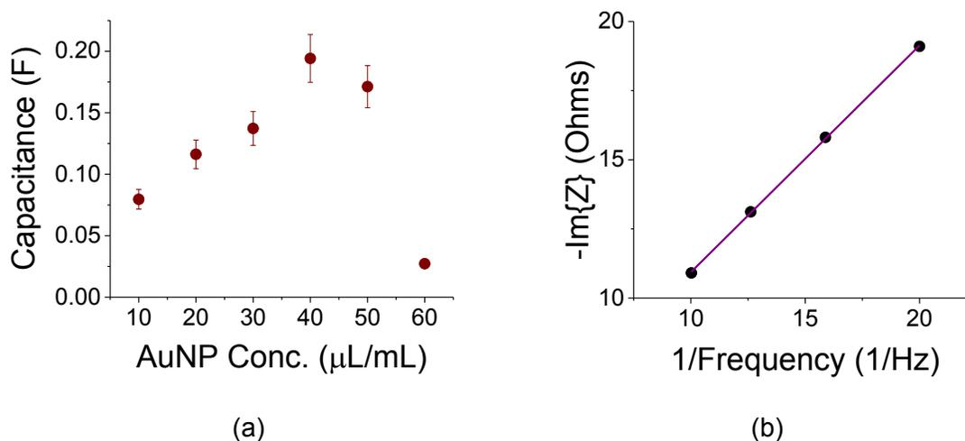
Figure 6. (a) Capacitance values, derived from EIS curves. The concentration of the AuNP is in mL per 1  $\mu\text{L}$  of solvent. (b) The slope of the linear curve for the sample exhibiting capacitance maxima at 40  $\mu\text{L}/\text{mL}$  of AuNPs is proportional to  $1/C_{\text{diff}}$ . The electrolyte was 1 M of Na<sub>2</sub>SO<sub>4</sub>.
