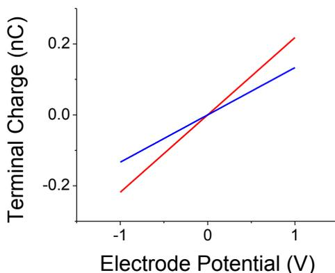
Figure 16. Change in electrode charge as a function of the bias,  $V_{in}$ . Blue line: graphite-like electrode without any colloid; Red line: graphite-like electrode with colloids on its surface. The cell capacitance is the slope of the linear Q-V curve.
