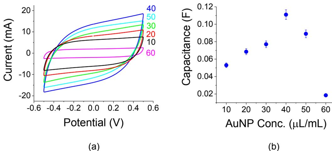
Figure 4. (a) Successive C-V plots for various concentrations (in  $\mu\text{L}$  per mL of solvent) depicted on the right. (b) Capacitance as a function of AuNPs concentration exhibits a peak at  $40 \mu\text{L}/\text{mL}$ . The electrolyte was 1 M of  $\text{Na}_2\text{SO}_4$ .
