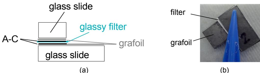
Figure 2. (a) A cross section of sample with grafoil coated active-carbon (A-C) electrodes, and (b) a picture of the cover area ca,  $1.27 \times 1.27 \text{ cm}^2$ .
