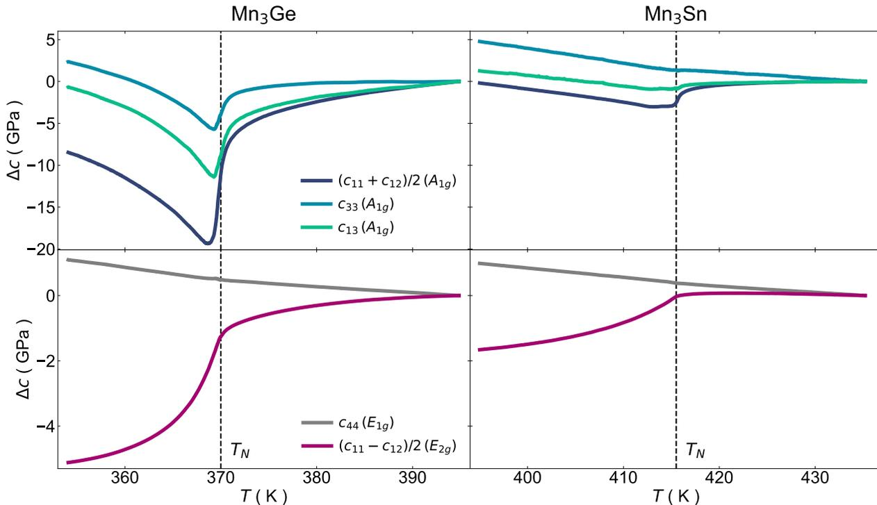
FIG. 2. **Change in elastic moduli as a function of temperature for Mn<sub>3</sub>Ge (left) and Mn<sub>3</sub>Sn (right)**. Upper and lower panels show elastic changes compressional and shear elastic moduli, respectively. The change is defined as  $\Delta c(T) = c(T) - c(387\text{K})$  for Mn<sub>3</sub>Ge and  $\Delta c(T) = c(T) - c(438\text{K})$  for Mn<sub>3</sub>Sn. The Néel temperatures are indicated by vertical dashed lines.
