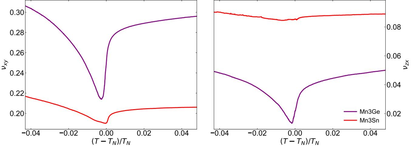
FIG. 7. We show the Poisson ratios  $\nu_{xy}$  (left panel) and  $\nu_{zx}$  for Mn<sub>3</sub>Ge (purple) and Mn<sub>3</sub>Sn (red) as a function of reduced temperature  $(T - T_N)/T_N$ . In a hexagonal crystal  $\nu_{zx} = \nu_{zy}$ .
