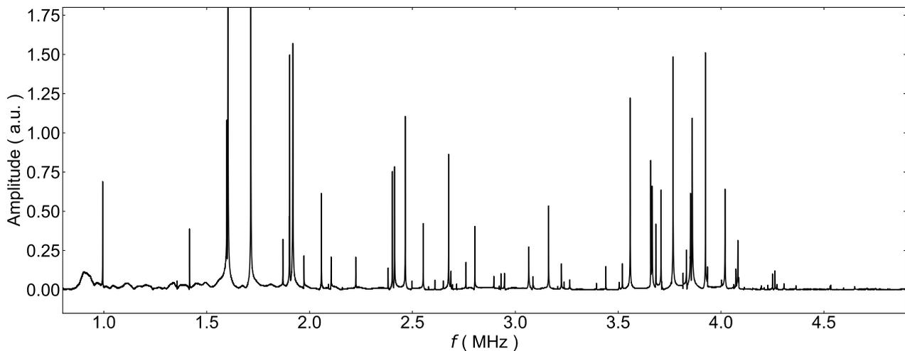
FIG. 6. Amplitude of the response of the receiving transducer in the RUS measurement of  $\text{Mn}_3\text{Sn}$  at room temperature.
