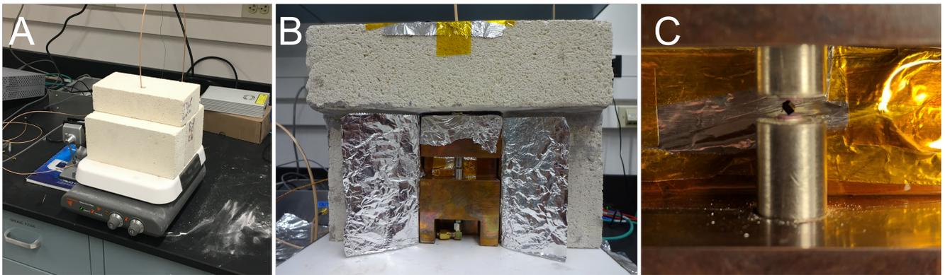
FIG. 5. Pictures of the custom-built high temperature RUS setup. Panel A) shows the entire setup covered by insulating firebricks. In panel B), one of the firebricks has been removed to give a better view of the copper mount. Panel C) shows a sample being mounted on its corners between two piezoelectric transducers.
