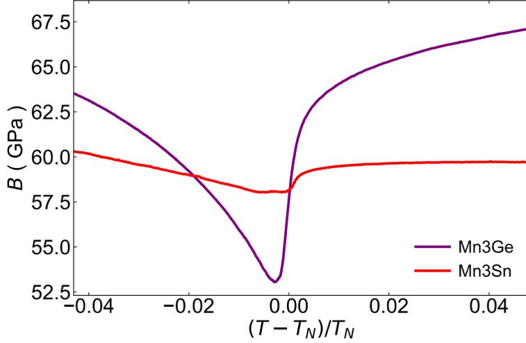
FIG. 8. We show the bulk moduli for Mn<sub>3</sub>Ge (purple) and Mn<sub>3</sub>Sn (red) as a function of reduced temperature  $(T - T_N)/T_N$ .
