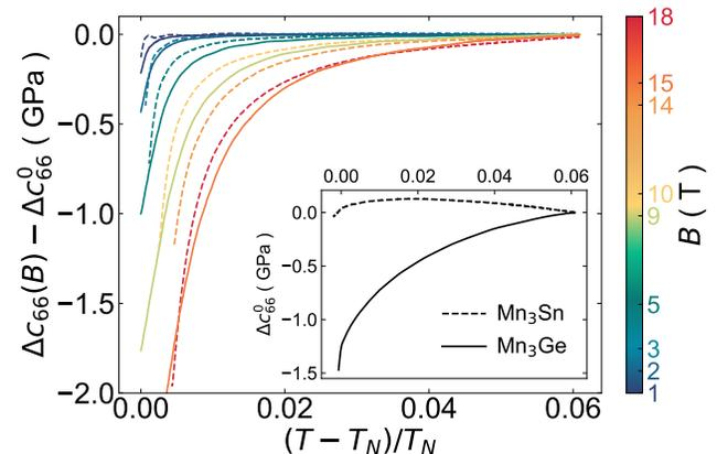
FIG. 4. **The field dependence of  $c_{66}$  in  $\text{Mn}_3\text{X}$ .** The changes in  $c_{66}$  for  $\text{Mn}_3\text{Ge}$  (solid lines) and  $\text{Mn}_3\text{Sn}$  (dashed lines) at different fields with respect to the zero-field elastic moduli are shown as a function of the reduced temperature. The data were taken at 1, 2, 5, 9, and 15 T for  $\text{Mn}_3\text{Ge}$  and at 1, 2.7, 5, 10, 14, and 18 T for  $\text{Mn}_3\text{Sn}$ . The inset shows the zero-field data for both compounds.
