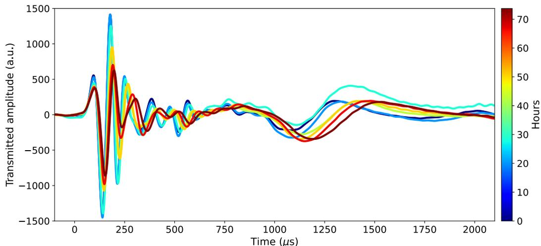
FIG. 2. Transmitted acoustic waves through a golden kiwifruit at  $\theta = 180^\circ$ , measured periodically over a range of 74 hours.
