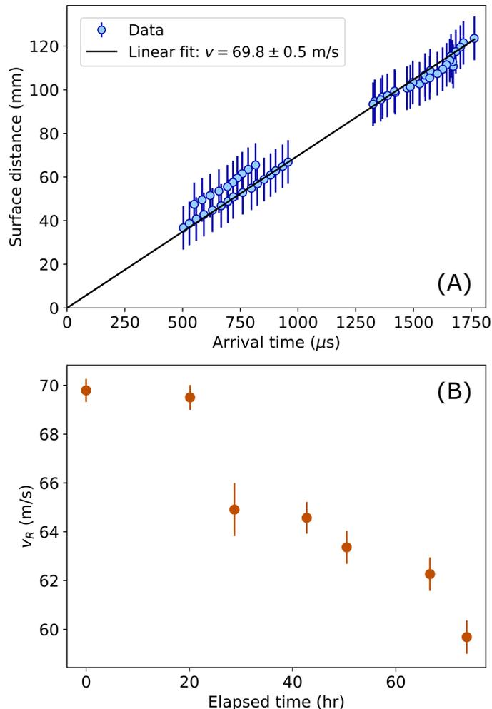
FIG. 3. (A) Experimentally-measured R-wave arrival times are plotted versus  $d_{\text{surface}}$ , distance travelled along the fruit surface from the source point (symbols). The slope of a linear fit (black line) gives an estimate of velocity  $v_R$ . Experimental data shown was measured after a time-lapse of 0 hours. (B) Results for  $v_R$  are shown for the entire time lapse period.
