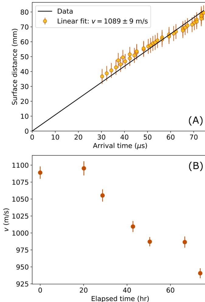
FIG. 4. (A) Experimentally-measured arrival times of the first-arriving wave are plotted versus  $d_{\text{surface}}$ , distance travelled along the fruit surface from the source point (symbols). Supposing that this wave is a surface wave, the slope of a linear fit (black line) gives an estimate of velocity  $v$ . Experimental data shown was measured after a time-lapse of 0 hours. (B) Results for  $v$  are shown for the entire time lapse period.
