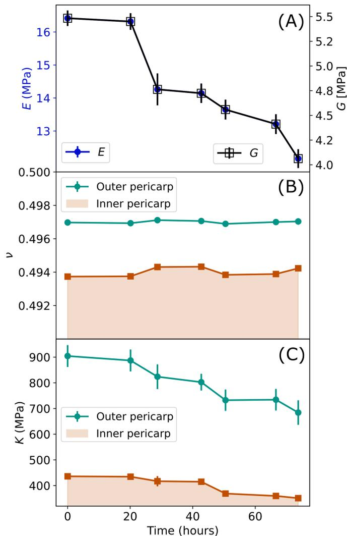
FIG. 6. Elastic wave parameters of a golden kiwifruit, measured over a time period of 74 hours. In (A)  $E$  and  $G$  in the outer pericarp are shown (values in the inner pericarp are identical, but constitute upper bounds). Values for (B)  $\nu$  and (C)  $K$  are shown for the outer pericarp (teal circular symbols) and inner pericarp (orange square symbols).
