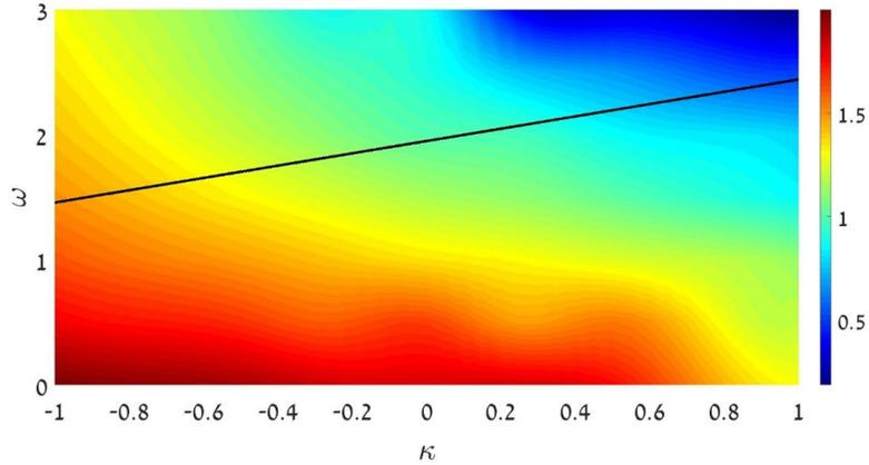
FIG. 5. The heatmap (gray-scale map, in the black-and-white rendition) of the eigenvalue of the 2D trapped state with  $S = 0$  (zero vorticity) in the  $(\kappa, \omega)$  plane at  $\lambda = 1$ , as produced by the numerical solution of the linearized equations (9) and (10). The black line represents relation (40), at which the exact 2D solution is given by Eqs. (35)-(39).
