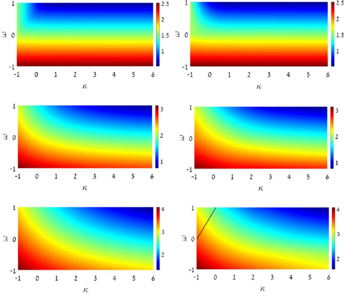
FIG. 4. Heatmaps (gray-scale maps, in the black-and-white rendition) of the DM eigenvalue in the  $(\kappa, \omega)$  planes, as produced by the numerical solution of the linearized equations (4) and (5), and by the VA (right and left panels, respectively). The top, middle, and bottom panels pertain to values of the coupling constant  $\lambda = 0.1, 1.0,$  and  $2.0$ . The black line in the right bottom panel represents relation (31), at which the exact solution is given by Eqs. (26)-(30).
