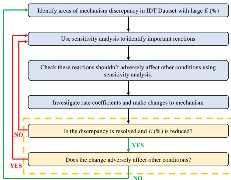
**Figure 9:** Modelling loop performed for the creation of the UoS sCO<sub>2</sub> mechanism.
