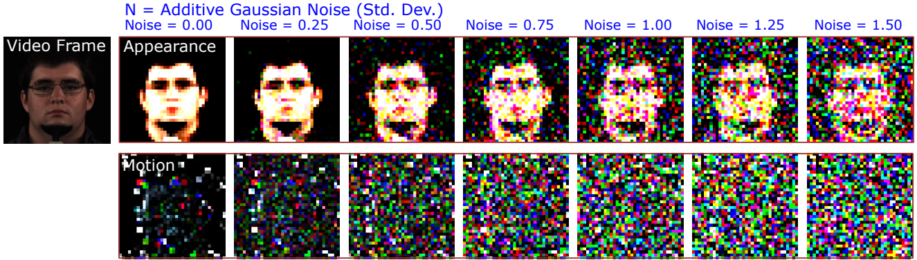
Figure 2. In our experiments we simulate camera sensor noise by adding Gaussian noise to the images. Here we illustrate the impact on the appearance and motion inputs to the two branch convolutional attention network.
