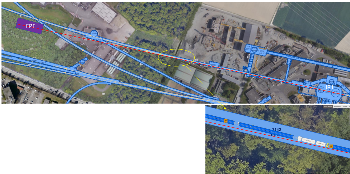
Figure 2.39: Plan view of the LHC complex between the ATLAS IP and the proposed FPF location. The LOS is shown as a red line, and the region where it has left the LHC magnet cryostats, but remains in the LHC tunnel, is highlighted in the zoomed in region. (Taken from the CERN GIS portal.)
