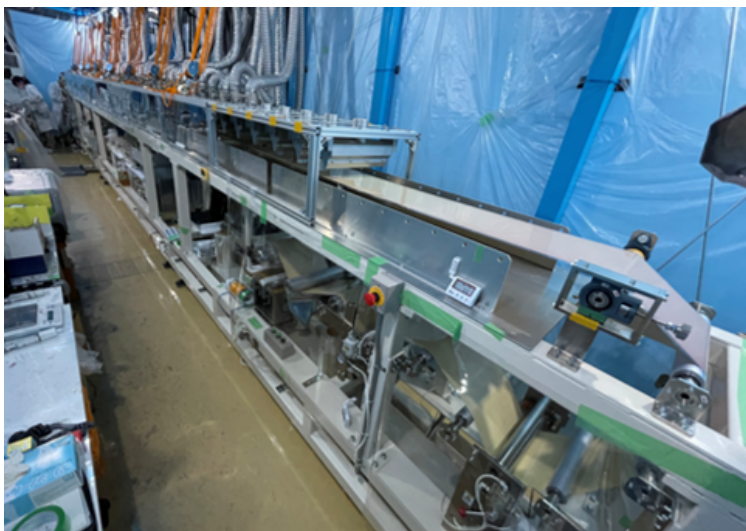
Figure 3.10: The emulsion film coating system.
