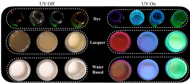
Fig. 2: **UV Paint Types:** We consider three types of UV-fluorescent paint in this paper: dyes (top), lacquer-based paint (middle), and water-based paints (bottom). We describe their properties and painting techniques in Section III-B. Most paints dry almost clear.
