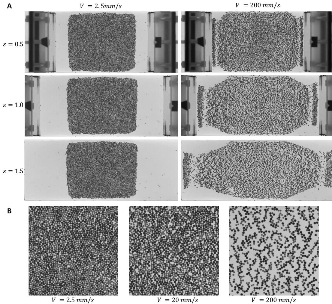
**Fig. 2** Failure morphology at different pulling speeds. (A) Snapshots of air-water experiments at different velocity,  $V$ , using repulsive boundary conditions. The series of images show the expansion of the rafts at low ( $V = 2.5 \text{ mm/s}$ ) and high ( $V = 200 \text{ mm/s}$ ) velocities. (B) Zoomed-in images show structure in the bulk of the rafts for a strain of  $\epsilon = 1.5$  at  $V = 2.5, 20, 200 \text{ mm/s}$  respectively.
