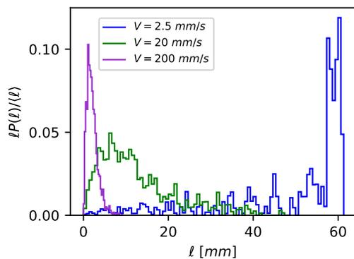
**Fig. 3** Distribution of cluster lengths,  $\ell$ , for different velocity at fixed strain in air-water experiments. The most dominant length, that is the probability of cluster length  $\ell$  multiplied by  $\ell$  normalized by  $\langle \ell \rangle = \Sigma \ell P(\ell)$ , is plotted versus  $\ell$  at a fixed strain  $\varepsilon = 1.0$  for three pulling speeds,  $V$ : 2.5 mm/s (blue), 20 mm/s (green) and 200 mm/s (purple).
